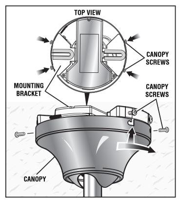
■ Lift the screw cover ring up over the screws and twist counterclockwise to secure in place.
