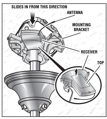
■ Slide the canopy up into place and rotate clockwise to lock to mounting bracket assembly. Reinstall the two screws (M4 x 6 mm) removed previously and tighten securely.
