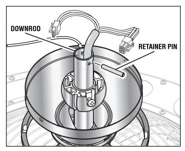
For Canada installations, refer to the Canada Installation Addendum and install the support cable on the retainer pin now.
