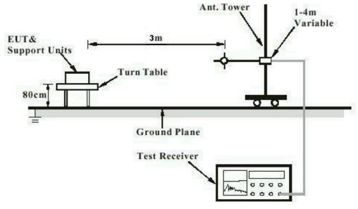
Note: Measurements above 1GHz are done with a table height of 1.5m. In addition, there is RF absorbing material on the floor of the test site for above 1GHz measurement.
