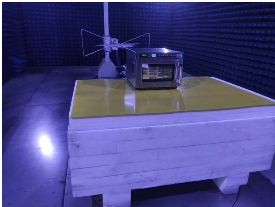
Photo of Radiated Emission Measurement Above 1GHz
