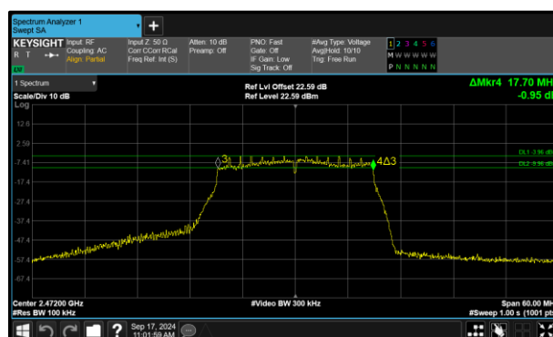
Figure 84 - 802.11n HT20 Maximum 6 dB EBW
