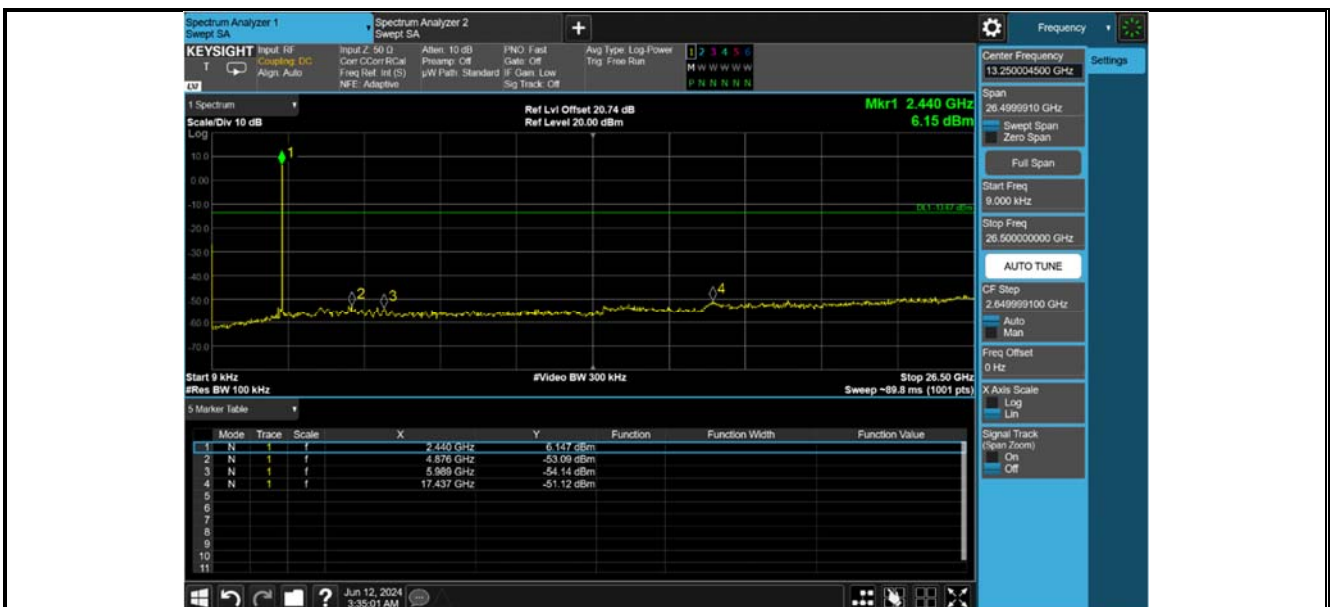
Mid Channel – 2440MHz Conducted Spurious Emission
