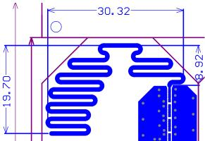
Antenna transmission frequency: 433.92MHz
