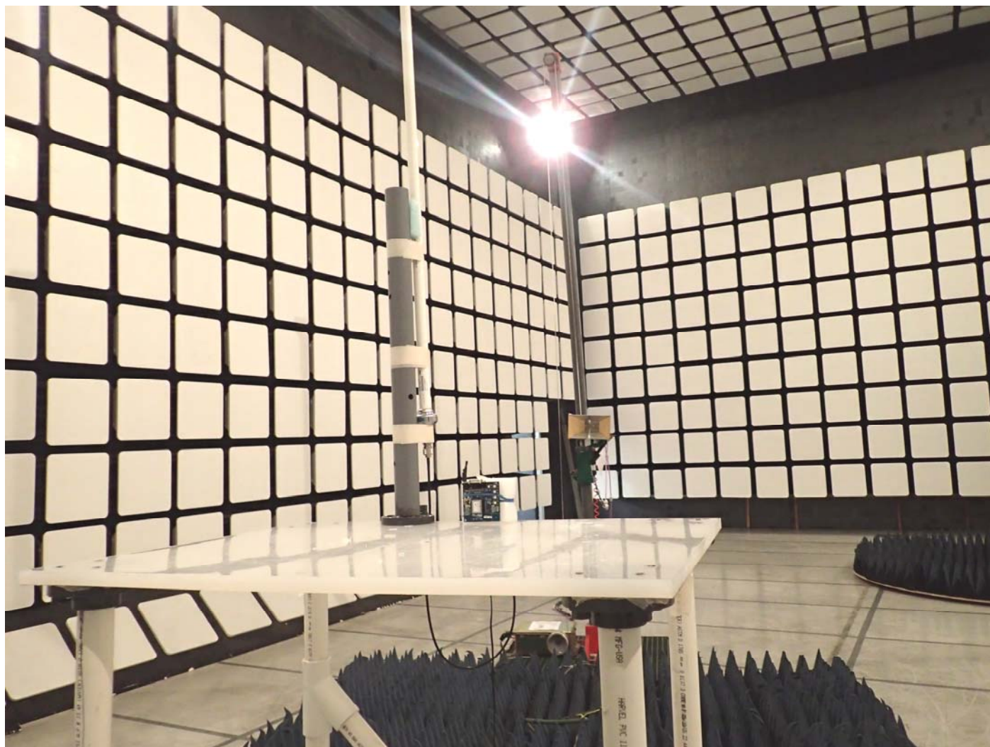
Radiated Emissions @ 3 m, Orthogonal Position 3 EUT with 15 dBi Omni-directional Antenna
