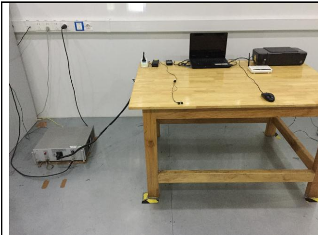
Conducted Emissions Test Setup – Front View
