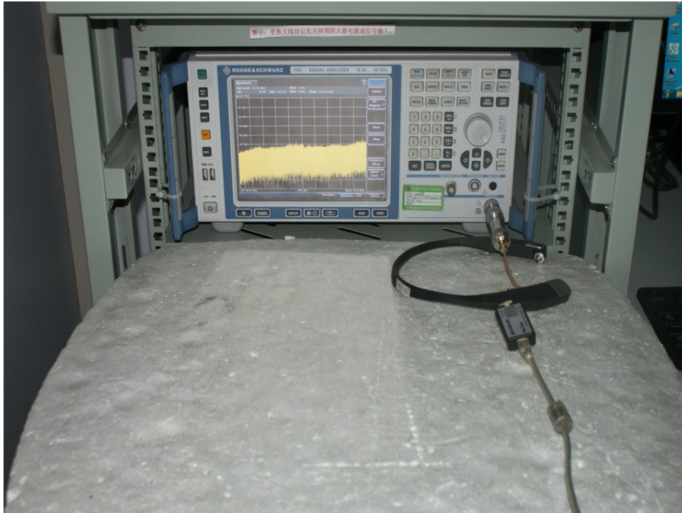
Photograph 2: Set-up for Spurious Emissions (9kHz-30MHz)
