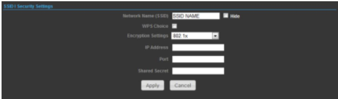
The screenshot shows the 'SSID Security Settings' interface. It includes a 'Network Name (SSID)' field with a 'Hide' checkbox, a 'WPS Choice' checkbox, an 'Encryption Settings' dropdown menu set to '802.1x', and input fields for 'IP Address', 'Port', and 'Shared Secret'. 'Apply' and 'Cancel' buttons are at the bottom.
