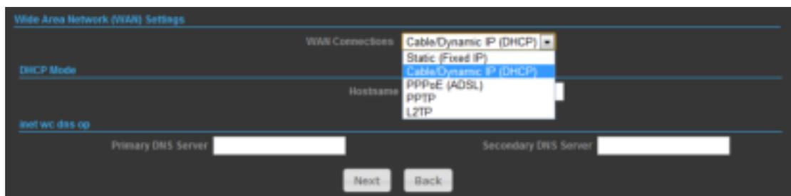
The screenshot shows the 'Wide Area Network (WAN) Settings' page. The 'WAN Connections' dropdown menu is open, displaying options: Cable/Dynamic IP (DHCP), Static (Fixed IP), Cable/Dynamic IP (DHCP) (highlighted), PPPoE (ADSL), pptp, and L2TP. Below the menu, there are fields for 'DHCP Mode', 'Hostname', 'Primary DNS Server', and 'Secondary DNS Server'. At the bottom, there are 'Next' and 'Back' buttons.
