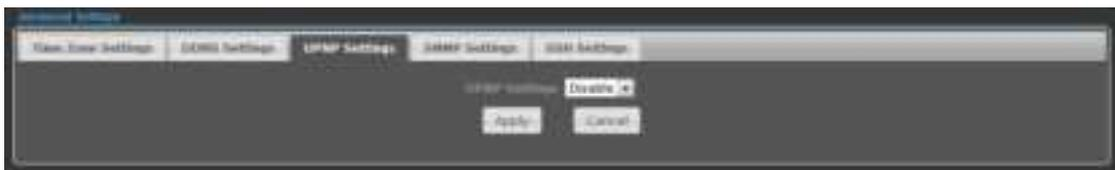
**UPnP Settings**— UPnP permits network devices to discover other network device(s) preference and establish functional network services for data sharing, communication, and entrainment. Default setting is Disabled.
