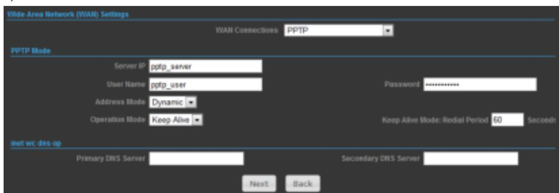
The screenshot shows the 'Wide Area Network (WAN) Settings' page with 'WAN Connections' set to 'PPTP'. The 'PPTP Mode' section includes fields for 'Server IP' (pptp\_server), 'User Name' (pptp\_user), 'Password' (masked), 'Address Mode' (Dynamic), 'Operation Mode' (Keep Alive), and 'Keep Alive Mode: Redial Period' (60 Seconds). Below these are fields for 'Primary DNS Server' and 'Secondary DNS Server'. At the bottom, there are 'Next' and 'Back' buttons.
