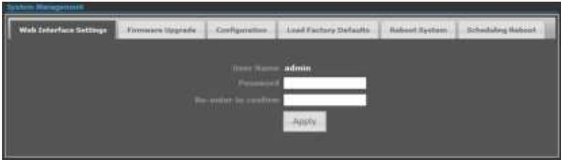
◆  **Password** — The new password must not exceed 32 characters in length and must not include any spaces. Enter the new password a second time to confirm it.
