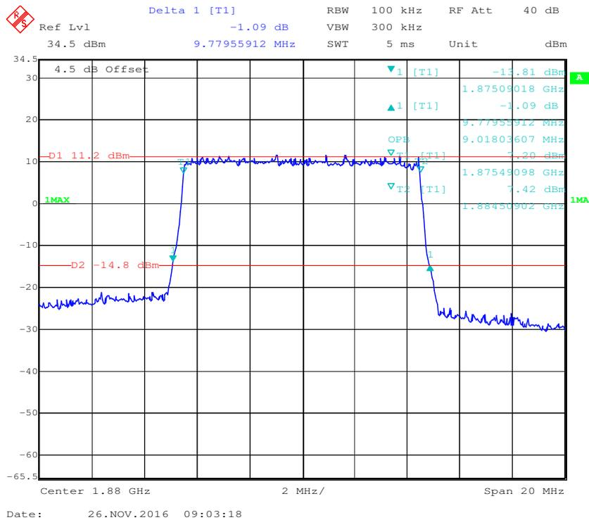
**QPSK (15.0 MHz) - 99% Occupied & 26 dB Emissions Bandwidth, Middle channel**
