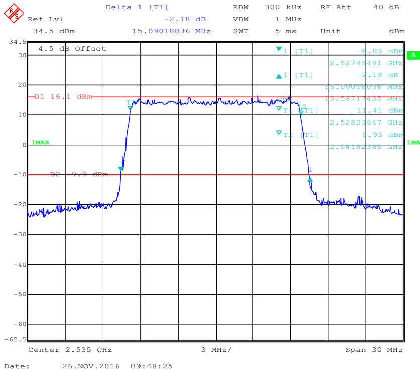
**16-QAM (15.0 MHz) - 99% Occupied & 26 dB Emissions Bandwidth, Middle channel**
