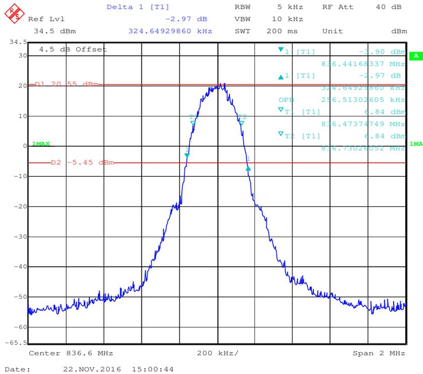
**26 dB Emissions & 99% Occupied Bandwidth for RMC (BPSK) Mode**
