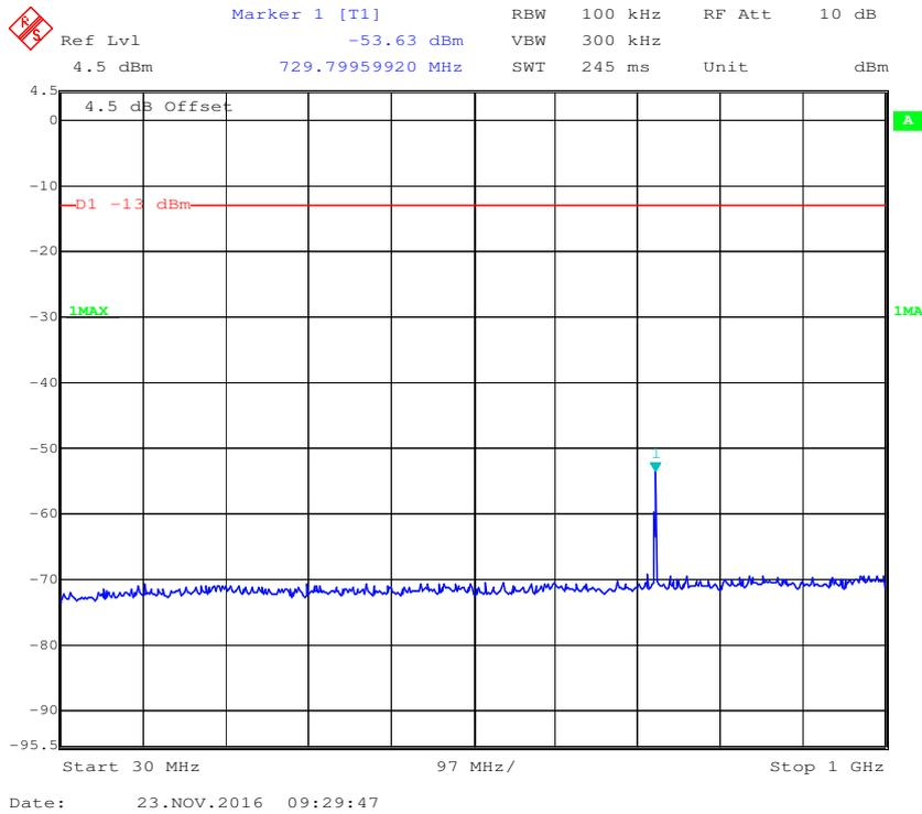
**1 GHz - 2 GHz (1.4 MHz, Middle Channel)**
