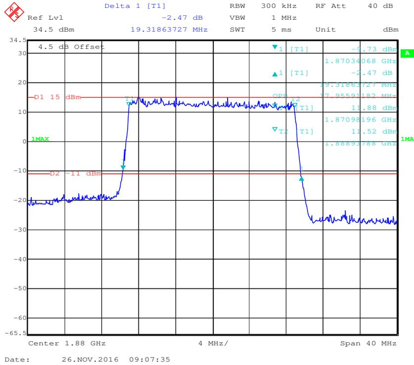
**16-QAM (20.0 MHz) - 99% Occupied & 26 dB Emissions Bandwidth, Middle channel**
