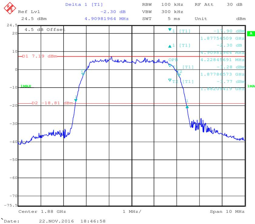
**26 dB Emissions & 99% Occupied Bandwidth for HSUPA (BPSK) Mode**
