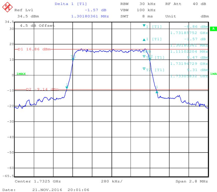
**QPSK (3.0 MHz) - 99% Occupied Bandwidth & 26 dB Bandwidth, Middle channel**
