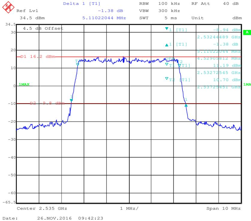
**16-QAM (5.0 MHz) - 99% Occupied & 26 dB Emissions Bandwidth, Middle channel**
