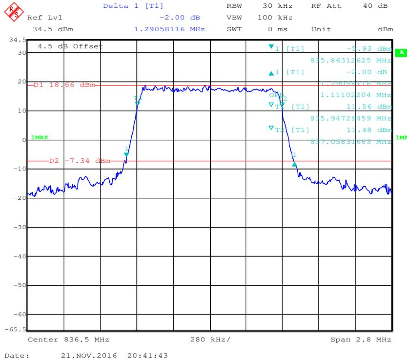
**16-QAM (1.4 MHz) - 99% Occupied Bandwidth & 26 dB Bandwidth, Middle channel**
