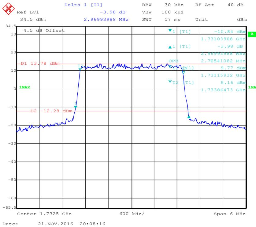
**QPSK (5.0 MHz) - 99% Occupied & 26 dB Emissions Bandwidth, Middle channel**
