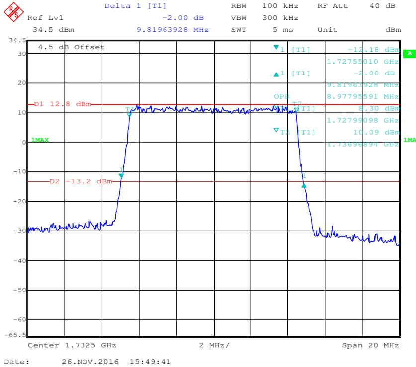
**16-QAM (10.0 MHz) - 99% Occupied & 26 dB Emissions Bandwidth, Middle channel**
