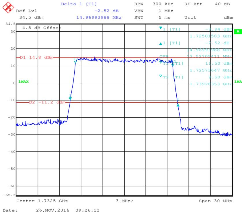
**QPSK (20.0 MHz) - 99% Occupied & 26 dB Emissions Bandwidth, Middle channel**
