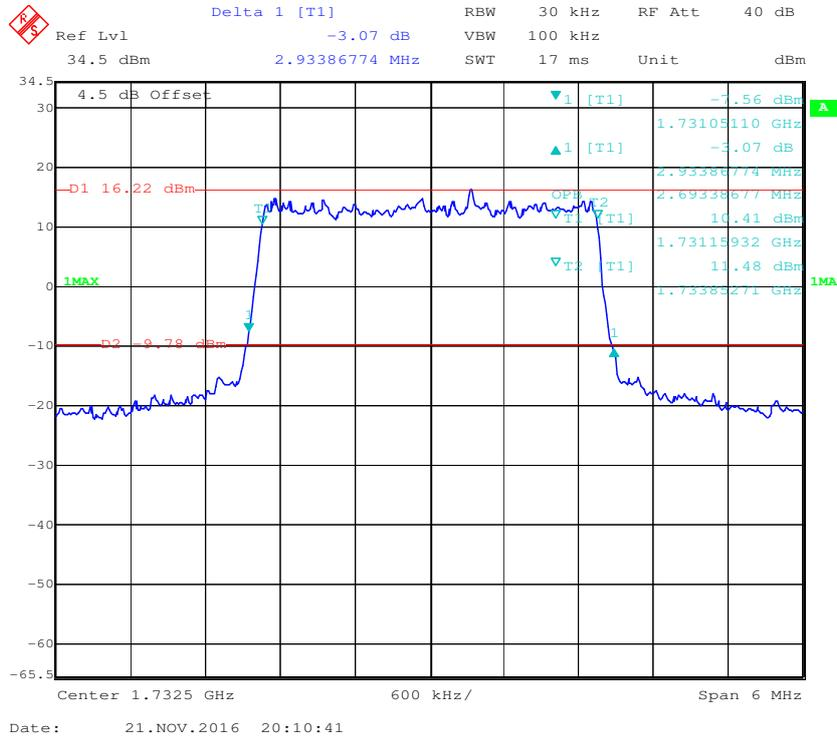
**16-QAM (3.0 MHz) - 99% Occupied Bandwidth & 26 dB Bandwidth, Middle channel**
