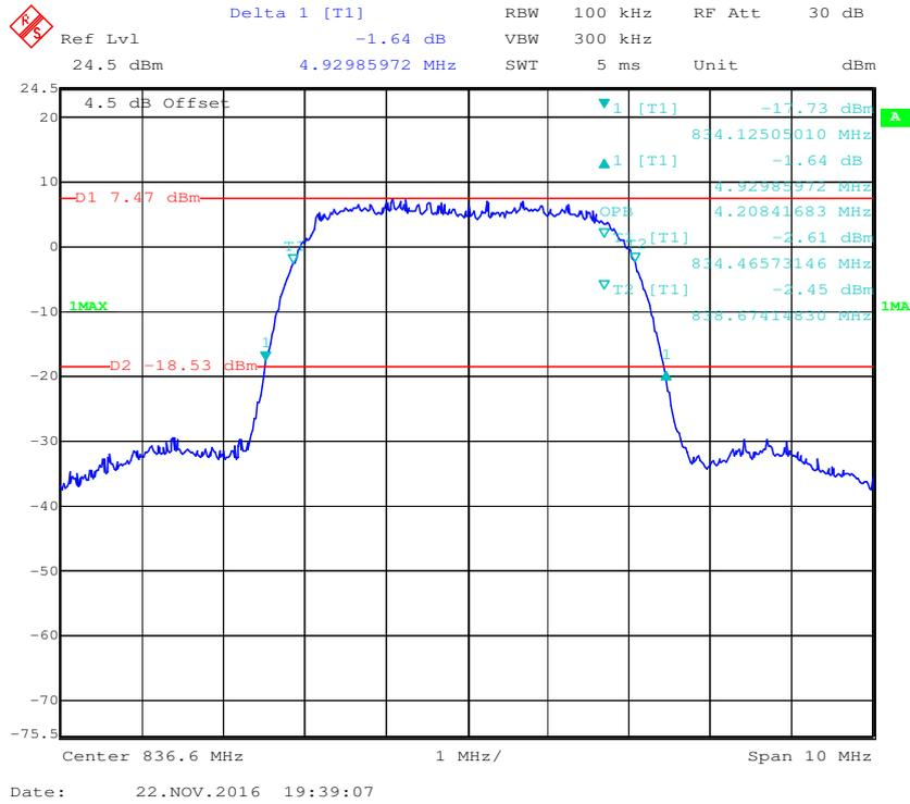
**26 dB Emissions & 99% Occupied Bandwidth for HSUPA (BPSK) Mode**
