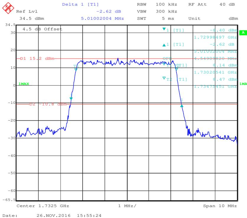
**QPSK (10.0 MHz) - 99% Occupied & 26 dB Emissions Bandwidth, Middle channel**
