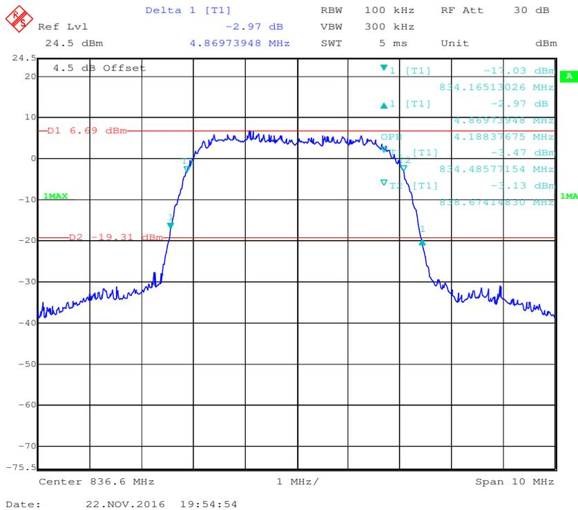
**26 dB Emissions & 99% Occupied Bandwidth for HSDPA (16QAM) Mode**
