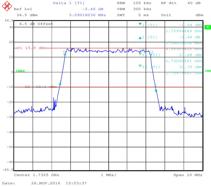
**16-QAM (5.0 MHz) - 99% Occupied & 26 dB Emissions Bandwidth, Middle channel**
