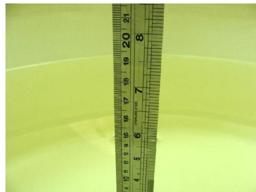
Fig 7.2 Photo of Liquid Height for Body SAR
