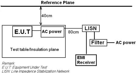
LISN: Line Impedence Stabiliz Test table height=0.8m
