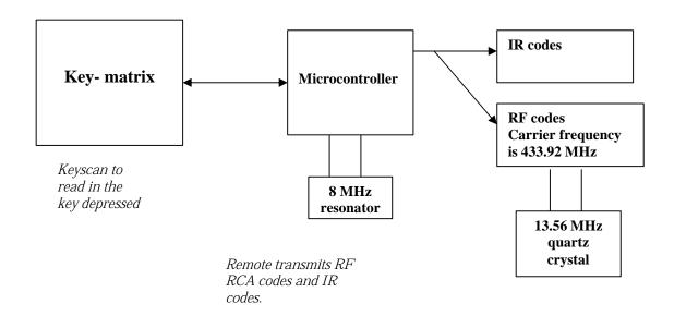
The RF codes are generated by modulating the RC codes with a 433.92 MHz RF IC which is present in the RF module.
