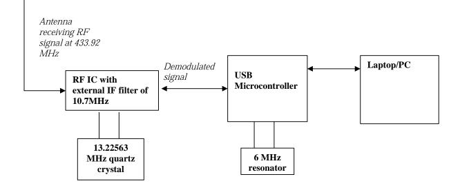
The RF IC receives the RF signal of 433.92MHz and the RF signal is mixed and demodulated to the baseband signal. The baseband signal is then sent to the USB microcontroller for communications with the PC/laptop.
