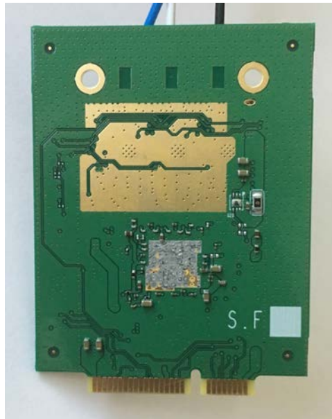
Figure 2 - 802.11bgn/Scanning WiFi Radio Module Bottom View
