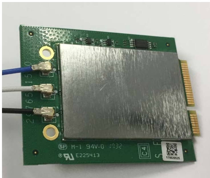
Figure 1 - 802.11bgn/Scanning WiFi Radio Module Front View
