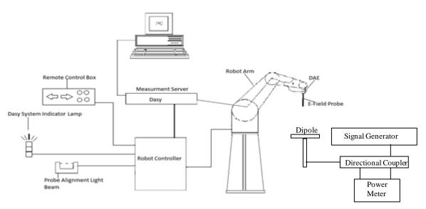
The Dasy5 HAC test system consists of:
