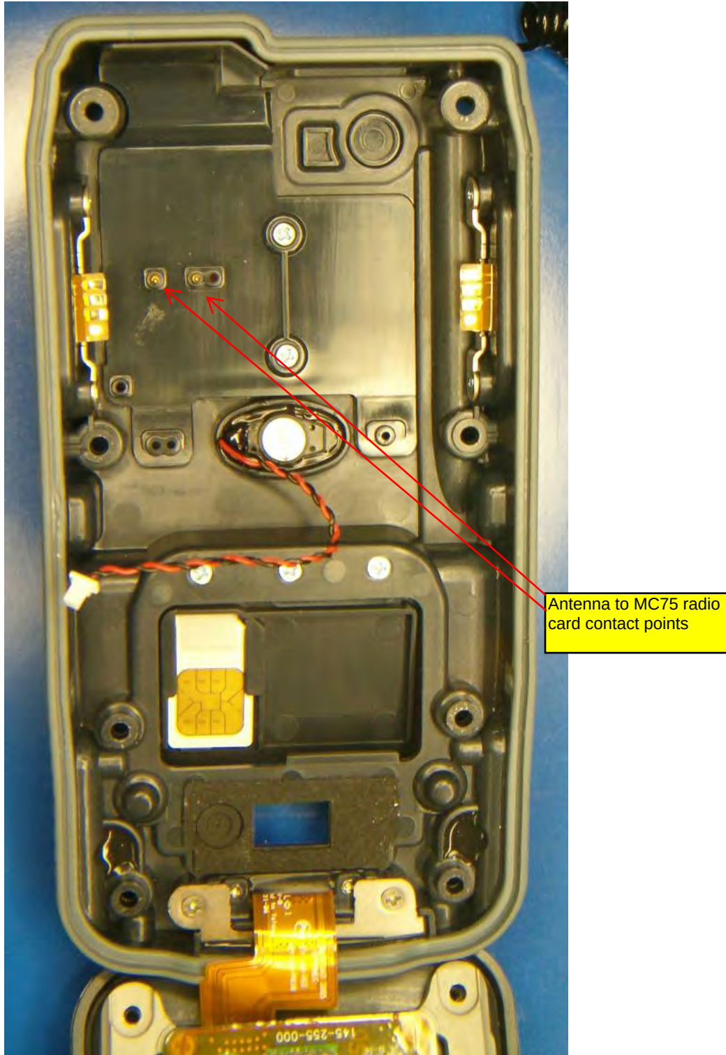
CN3 Case Back with MC75 Antenna Installed
