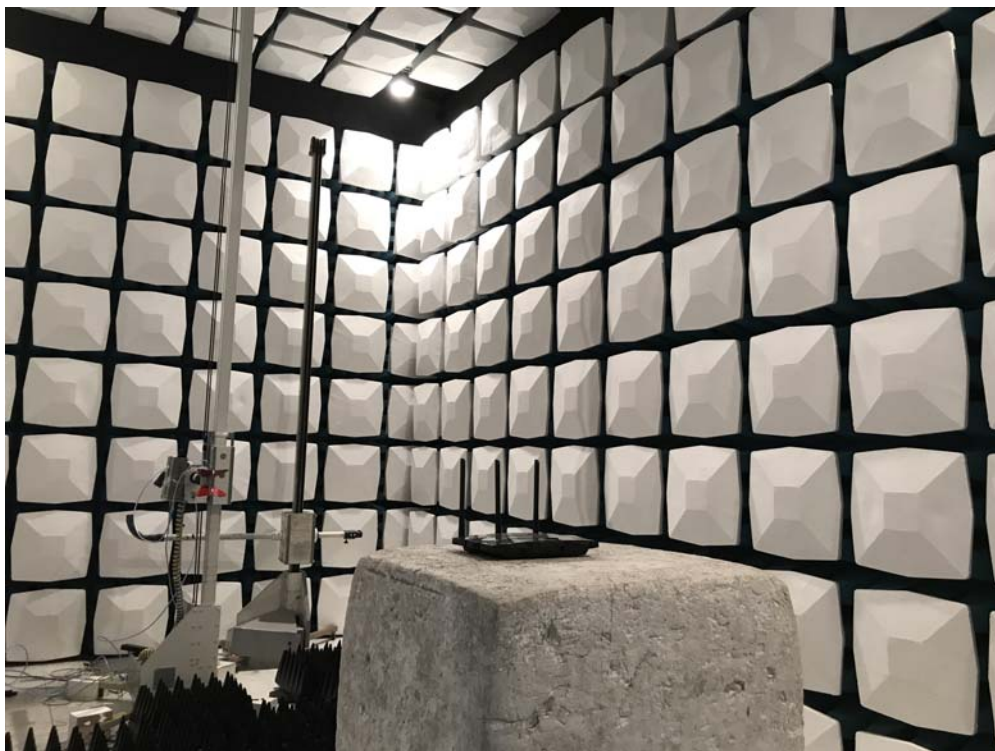
Description: Radiated Emission Test Setup for 1~18GHz
