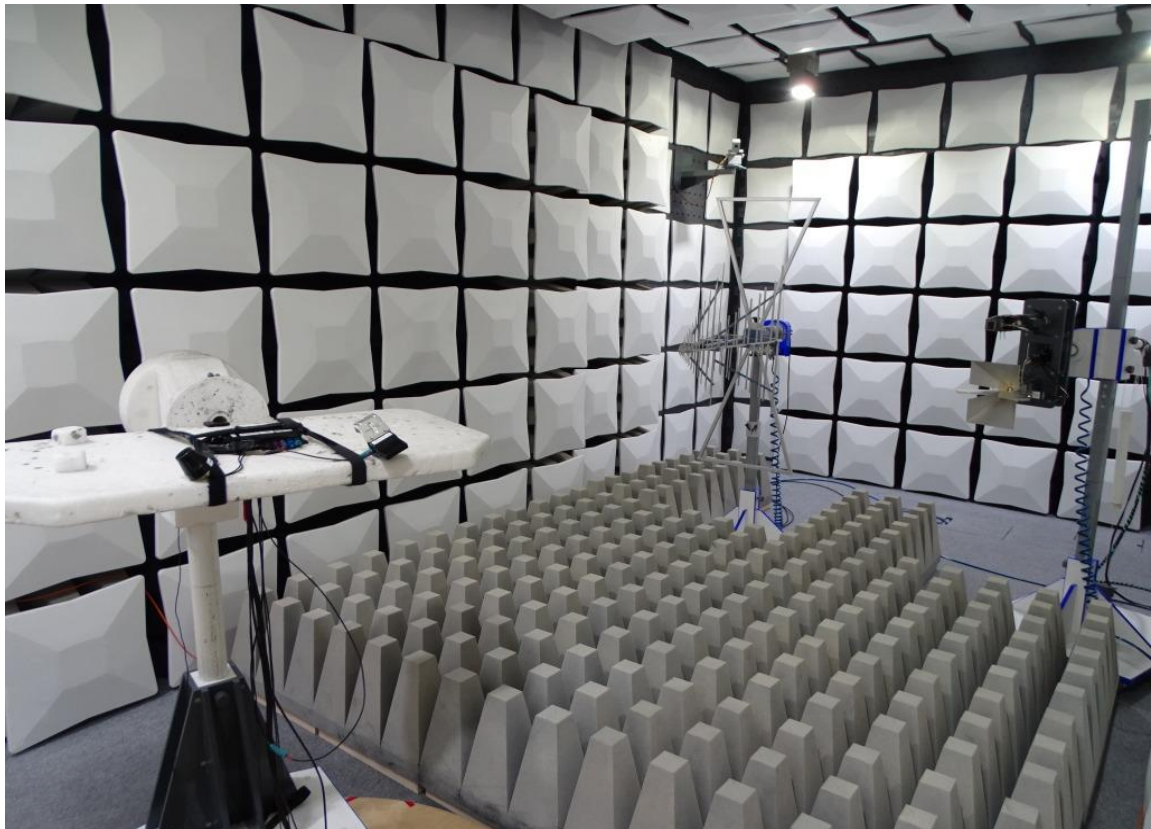
Photo 3: Test setup for radiated measurements above 1 GHz
