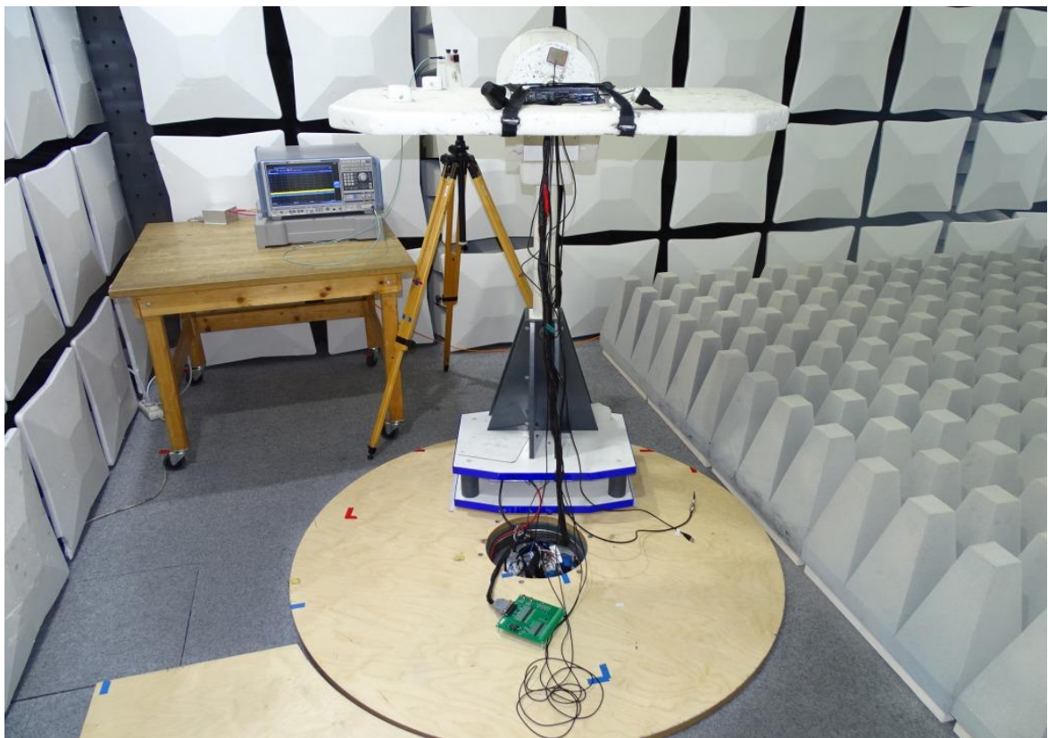
Photo 4: Test setup for radiated measurements above 26 GHz
