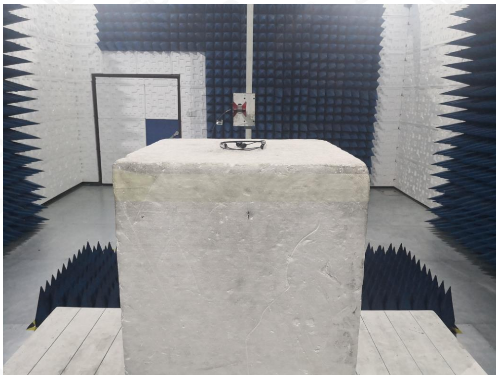
RADIATED EMISSION TEST SETUP ABOVE 1GHZ
