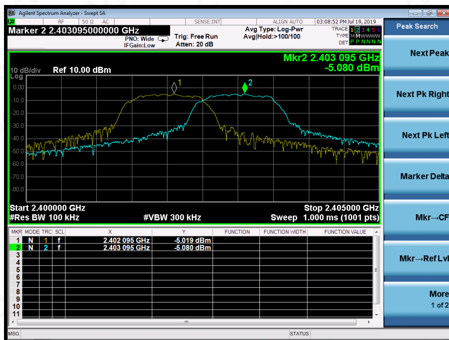
TEST PLOT FOR FREQUENCY SEPARATION
