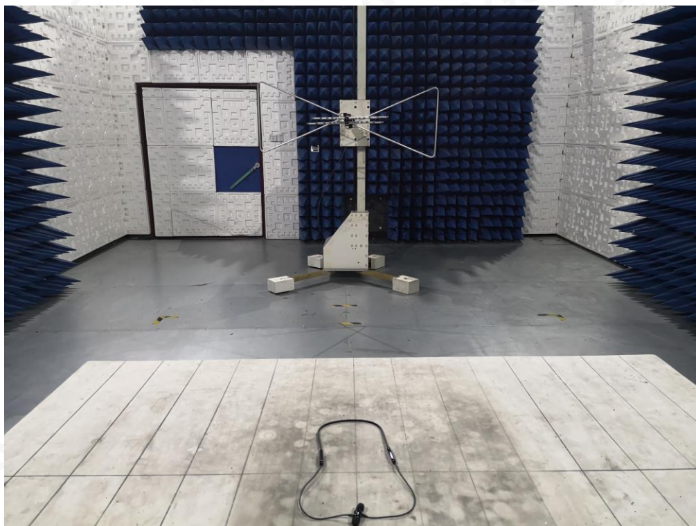
RADIATED EMISSION TEST SETUP ABOVE 1GHZ
