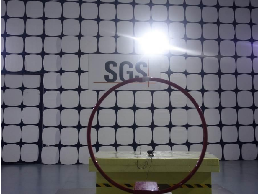
Radiated Emissions (9kHz-30MHz)
