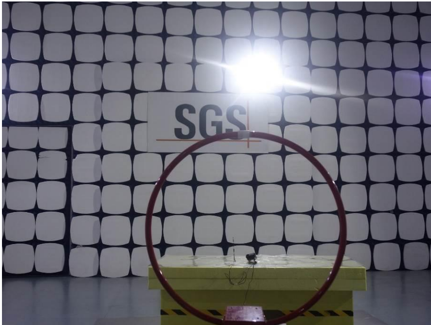
Radiated Emissions (9kHz-30MHz)
