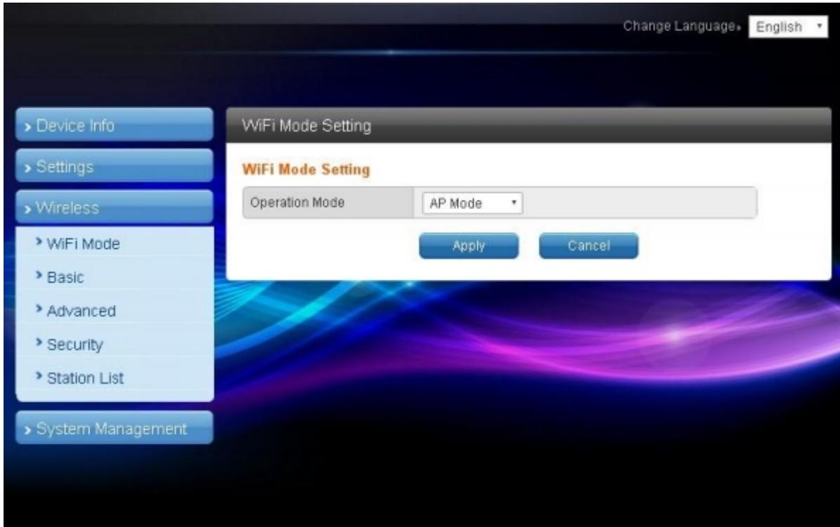
You may set WiFi mode into "Wireless AP mode" and "Wireless client mode". The wireless AP mode is an AP with gateway serving as WiFi access point.
