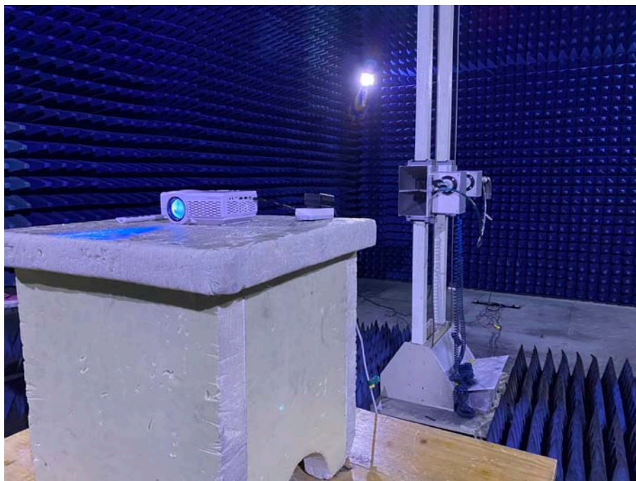
Photo of Radiated Emission Measurement (Above 1G)
