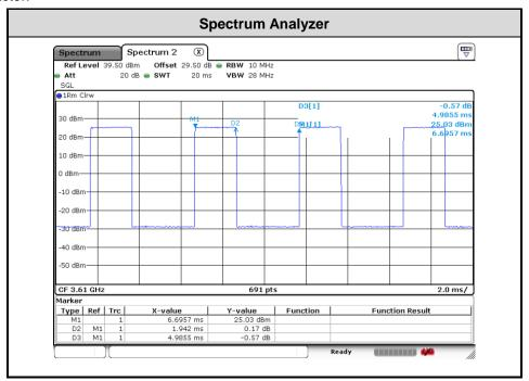
Note: The duty cycle value is 38.953%, add 10log(1/duty cycle) to the measured power level to compute the average power during continuous transmission.
