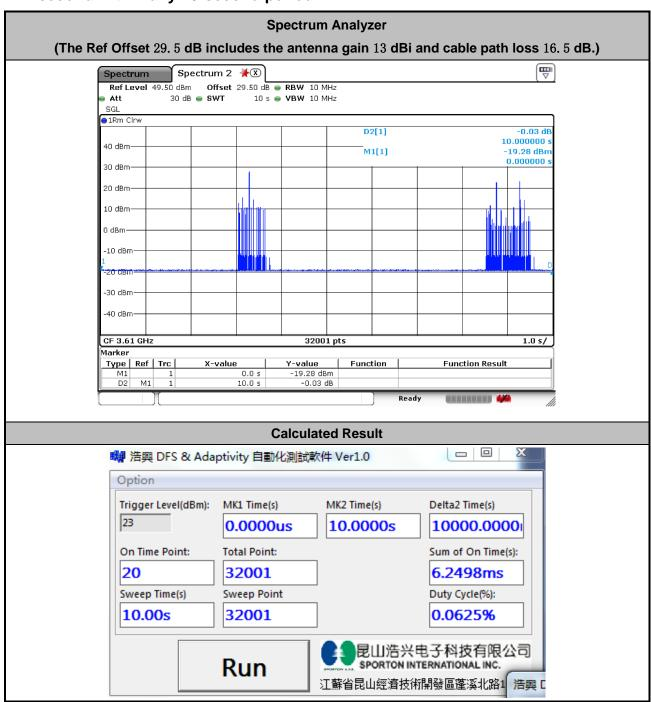
The sum of On Time (aggregated time from marker 1 to 2): 6.2498ms < 1s, Pass.
