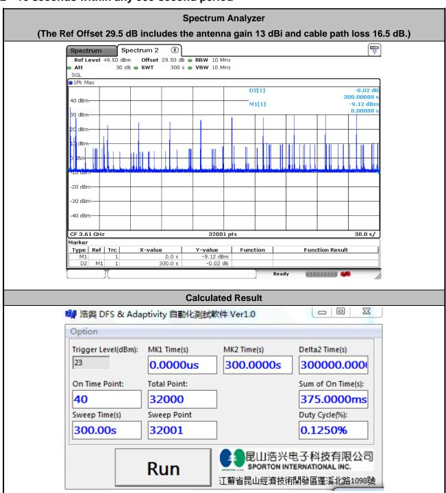
The sum of On Time (aggregated time from marker 1 to 2): 375ms < 10s, Pass.
