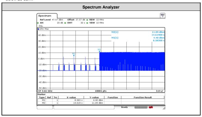
Note: The Ref Offset 37.57 dB includes the antenna gain 13 dBi and cable path loss 24.57dB.
