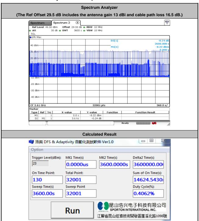
The sum of On Time (aggregated time from marker 1 to 2): 14624.543ms < 20s, Pass.
