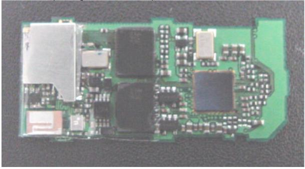
CJ6SD00UBT Front PCB view without shielding on Bluetooth Module:
