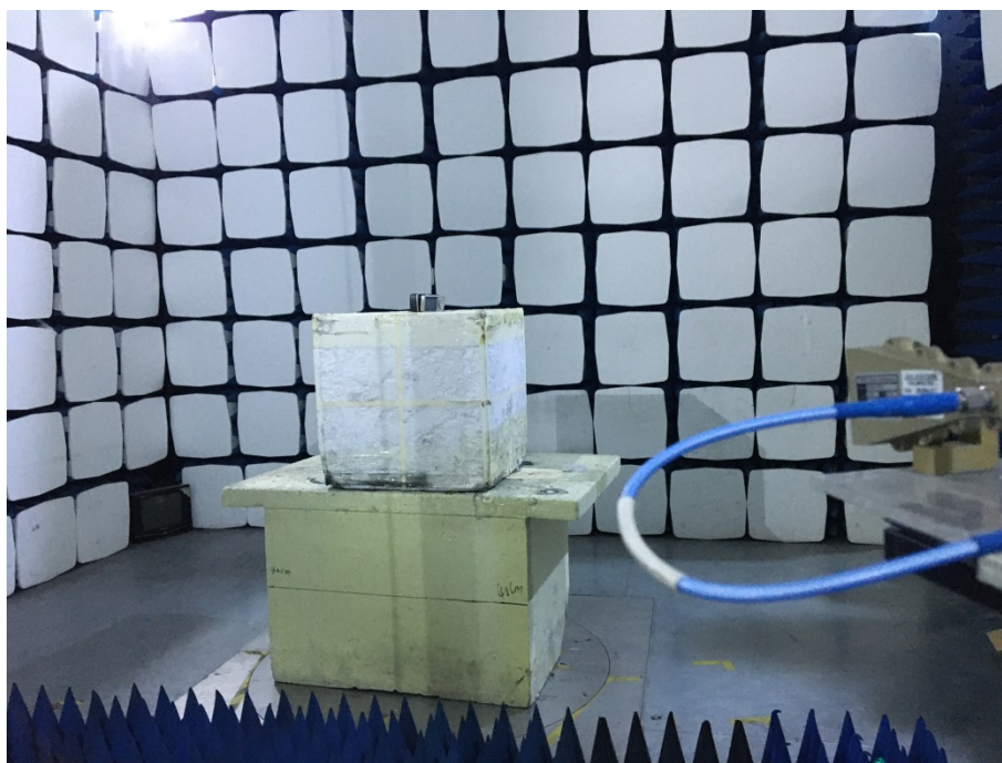
Radiation Emission Test Setup (Above 18GHz)
