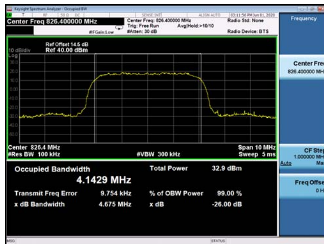
(Plot E1: WCDMA 850MHz Channel = 4132 Occupied bandwidth)
