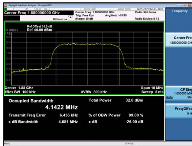
(Plot F2: WCDMA 1900MHz Channel = 9400 Occupied bandwidth)
