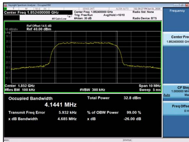
(Plot F1: WCDMA 1900MHz Channel = 9262 Occupied bandwidth)
