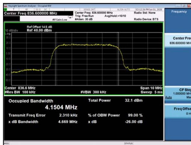
(Plot E2: WCDMA 850MHz Channel = 4183 Occupied bandwidth)
