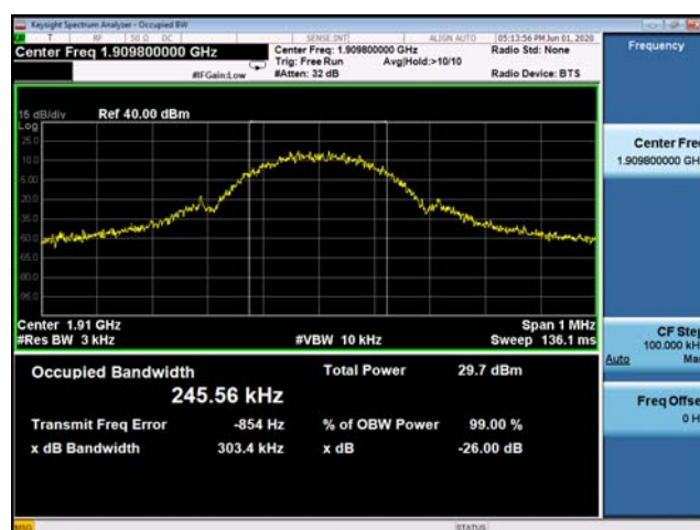
(Plot B3: GSM 1900MHz Channel = 810 Occupied bandwidth)
