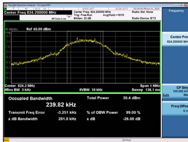
(Plot C1: EDGE 850MHz Channel = 128 Occupied bandwidth)
