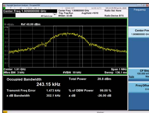
(Plot D3: EDGE 1900MHz Channel = 810 Occupied bandwidth)
