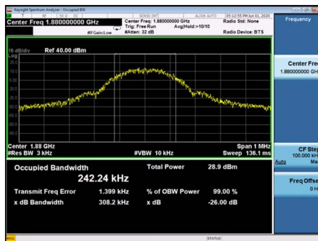
(Plot D2: EDGE 1900MHz Channel = 661 Occupied bandwidth)
