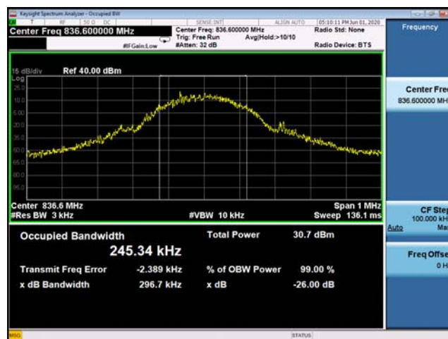
(Plot C2: EDGE 850MHz Channel = 190 Occupied bandwidth)
