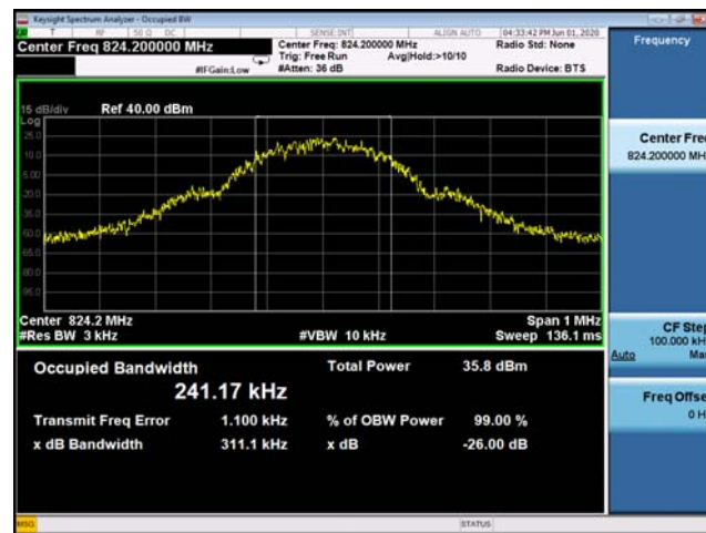
(Plot A1: GSM 850MHz Channel = 128 Occupied bandwidth)
