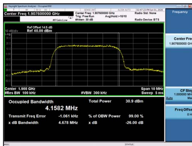
(Plot F3: WCDMA 1900MHz Channel = 9538 Occupied bandwidth)
