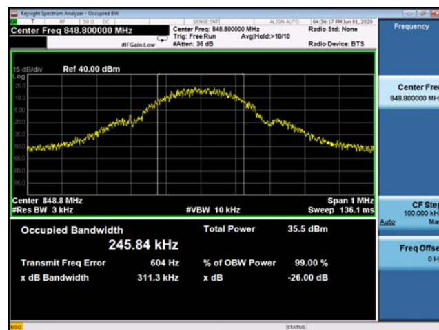
(Plot A3: GSM 850MHz Channel = 251 Occupied bandwidth)
