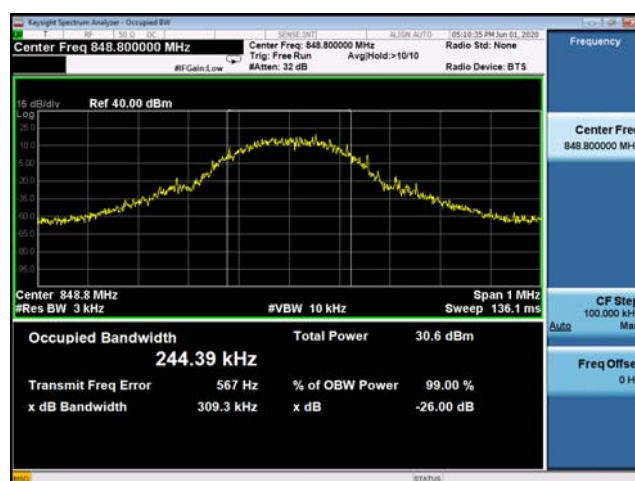
(Plot C3: EDGE 850MHz Channel = 251 Occupied bandwidth)
