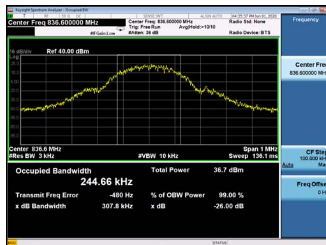
(Plot A2: GSM 850MHz Channel = 190 Occupied bandwidth)
