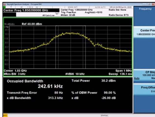
(Plot D1: EDGE 1900MHz Channel = 512 Occupied bandwidth)
