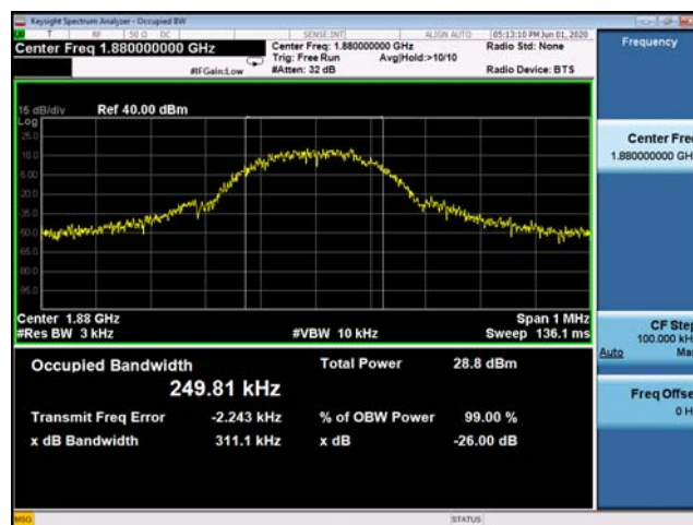
(Plot B2: GSM 1900MHz Channel = 661 Occupied bandwidth)
