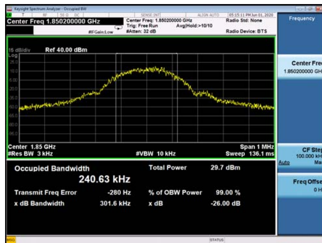
(Plot B1: GSM 1900MHz Channel = 512 Occupied bandwidth)
