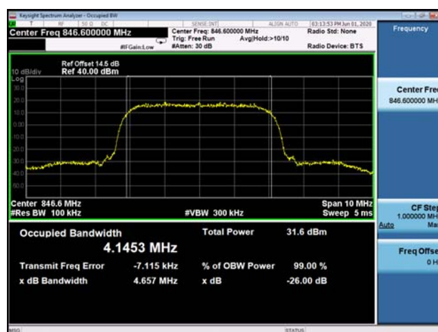
(Plot E3: WCDMA 850MHz Channel = 4233 Occupied bandwidth)
