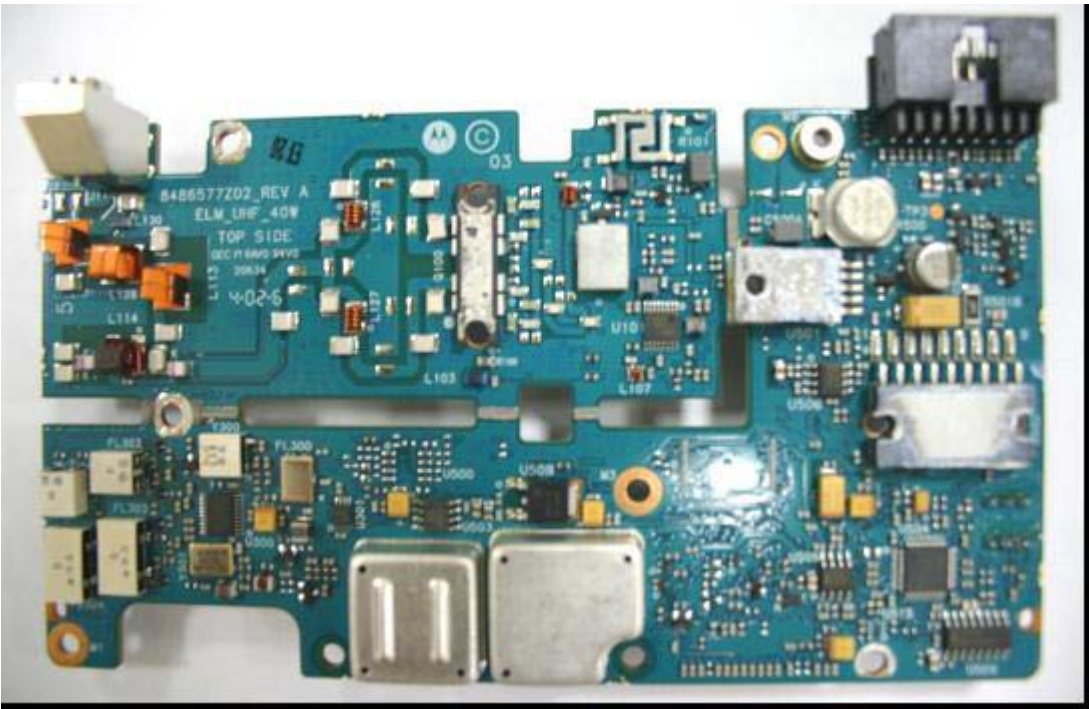
Figure 9-3: Top Side of PCB with shields.
