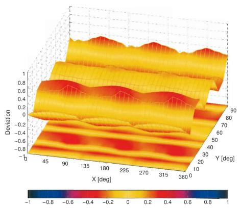
Probe isotropy for E<sub>tot</sub>: probe rotated  $\phi=0^\circ$  to 360°, tilted from field propagation direction  $\vec{k}$  Parallel to the field propagation ( $\psi=0^\circ-90^\circ$ ) at 30 GHz: deviation within  $\pm 0.33$  dB Parallel to the field propagation ( $\psi=0^\circ-90^\circ$ ) at 60 GHz: deviation within  $\pm 0.38$  dB
