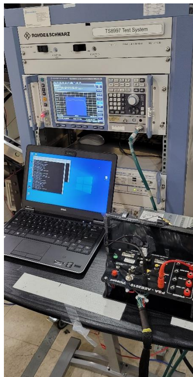
Figure B4. Conducted test setup
