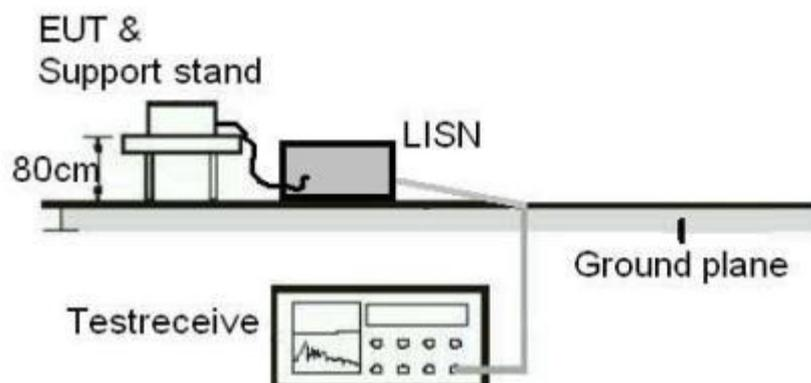
**Diagram of Measurement Configuration for Conducted Transmitter Measurement**
