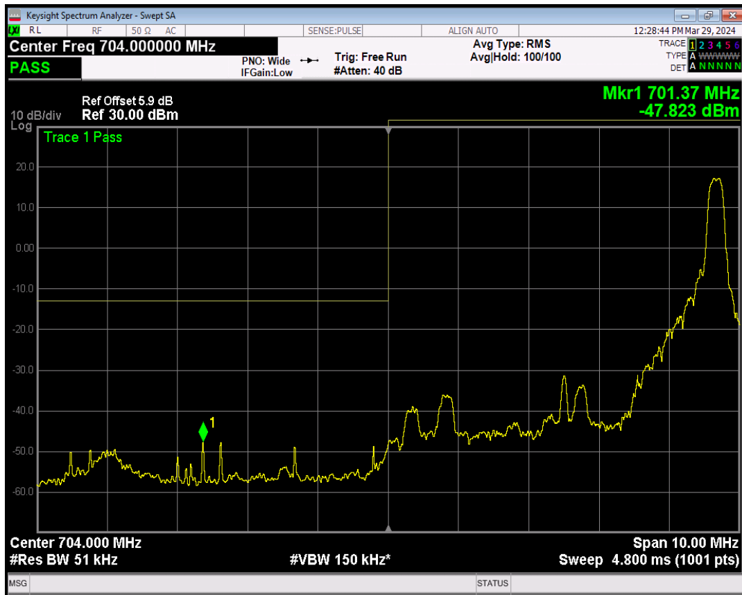
Band17 QPSK BW=5MHz Channel=23755 RB Size=25 Position=#0
