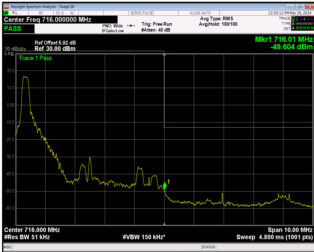
Band17 16QAM BW=5MHz Channel=23825 RB Size=1 Position=#Max
