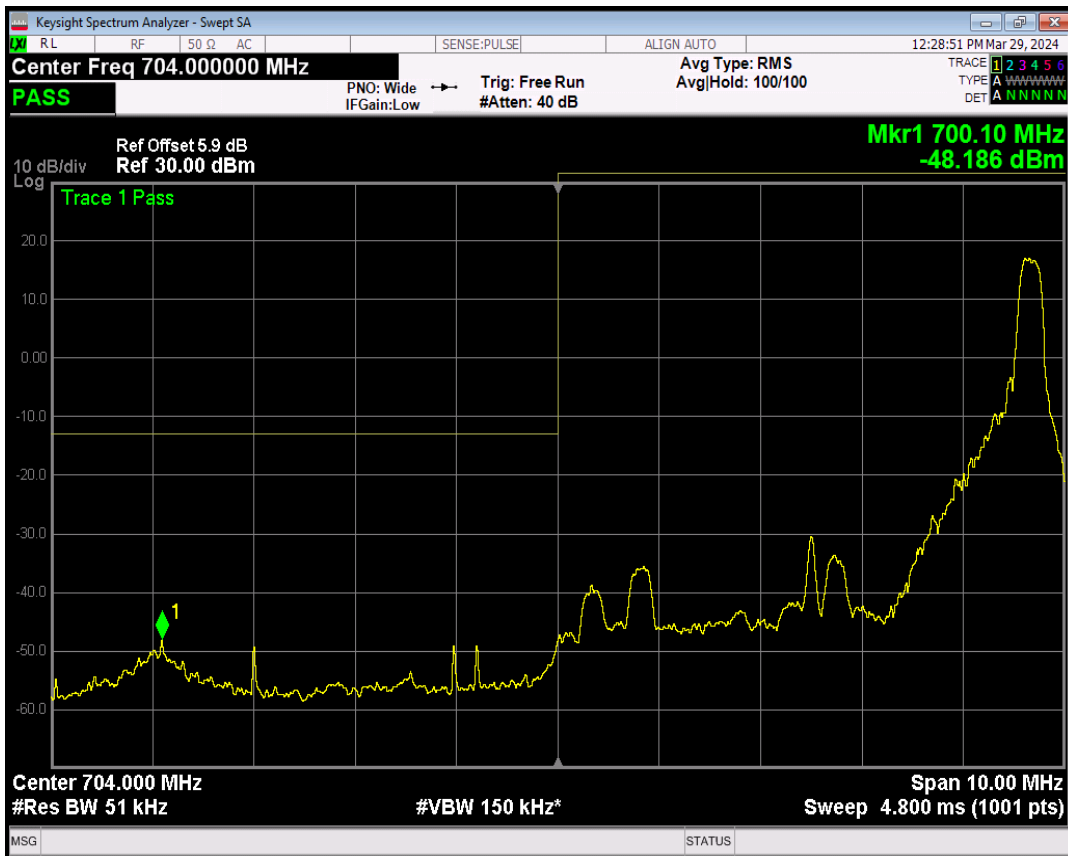
Band17 16QAM BW=5MHz Channel=23755 RB Size=25 Position=#0
