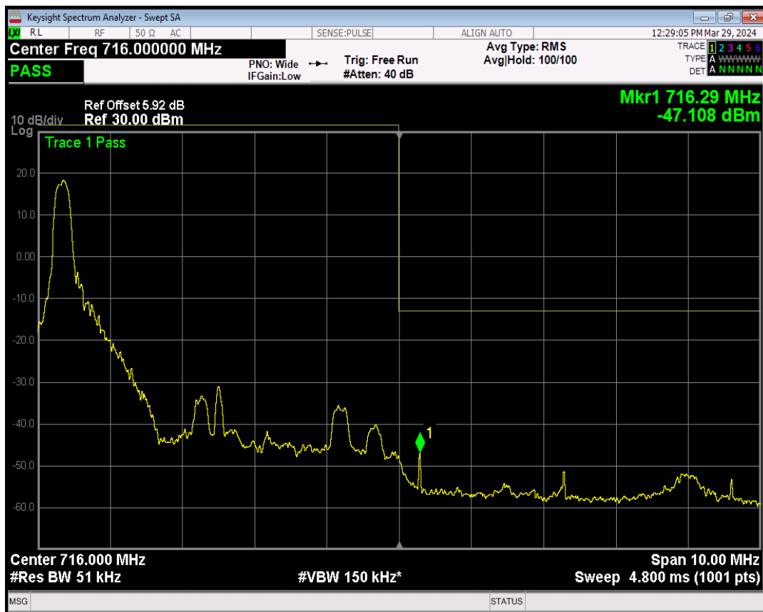
Band17 QPSK BW=5MHz Channel=23825 RB Size=1 Position=#Max
