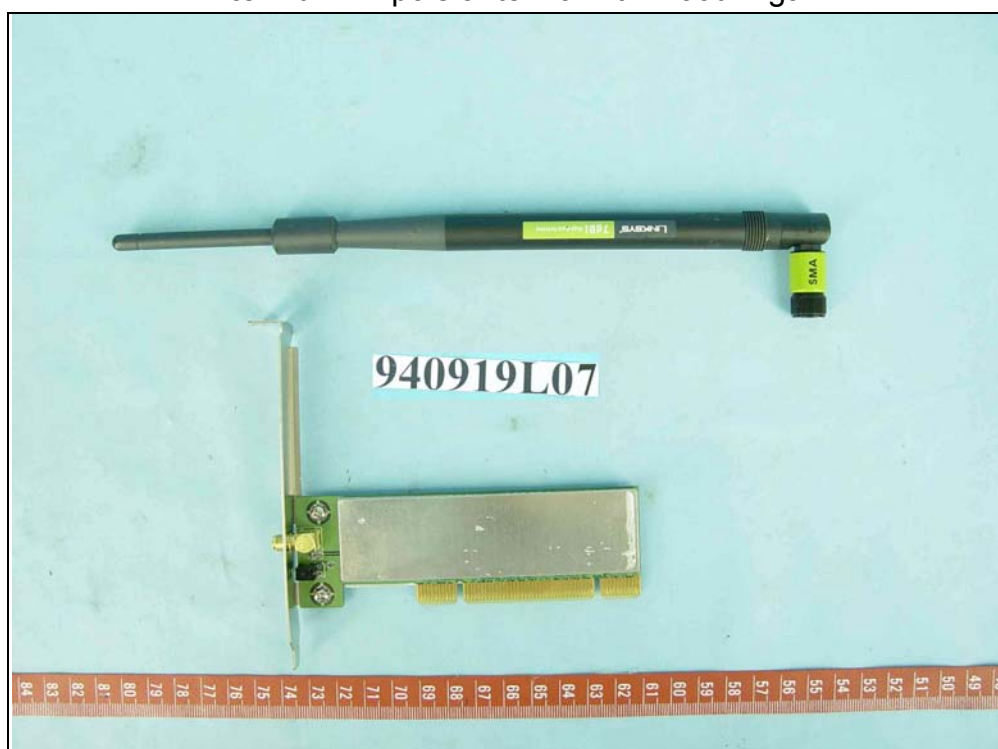
Antenna 2: Dipole antenna with 7.00dBi gain
