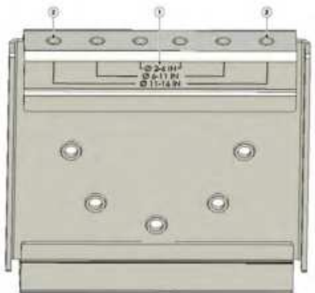
Figure 20: Pole Clamp Bracket Adjustment Hole Locations
