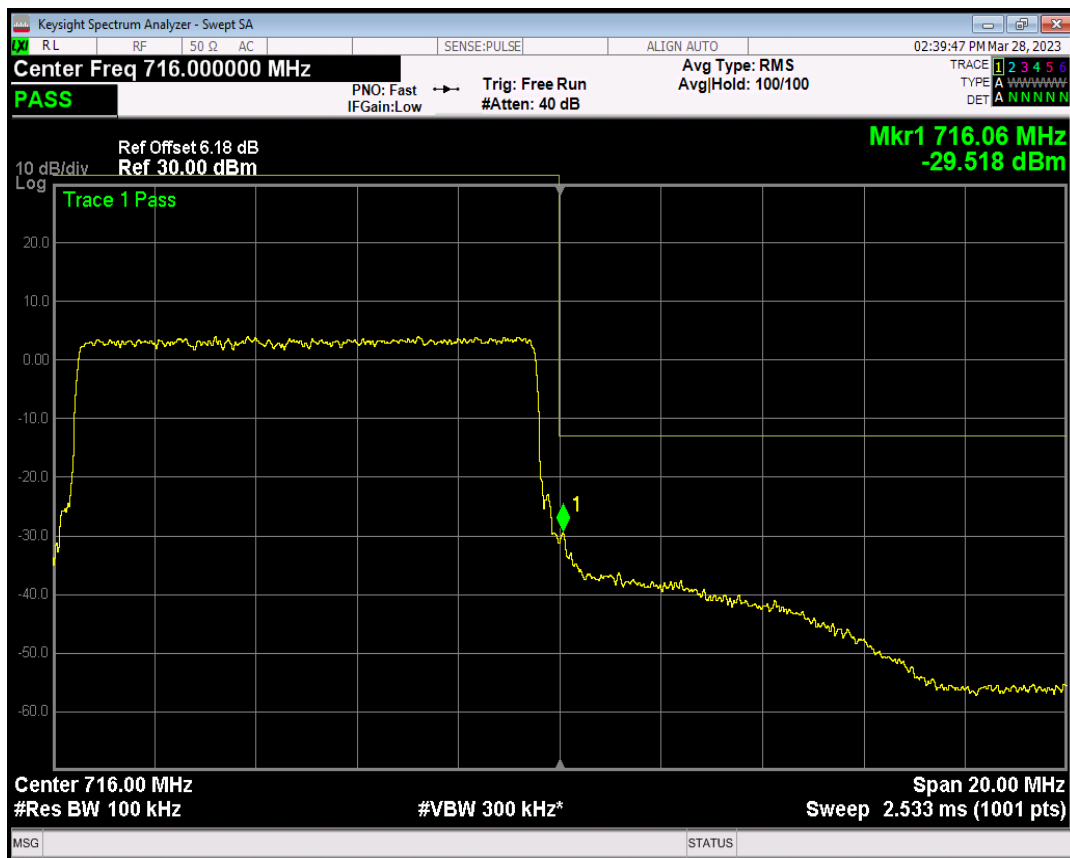
Band17 QAM16 BW=10MHz Channel=23800 RB Size=1 Position=#0
