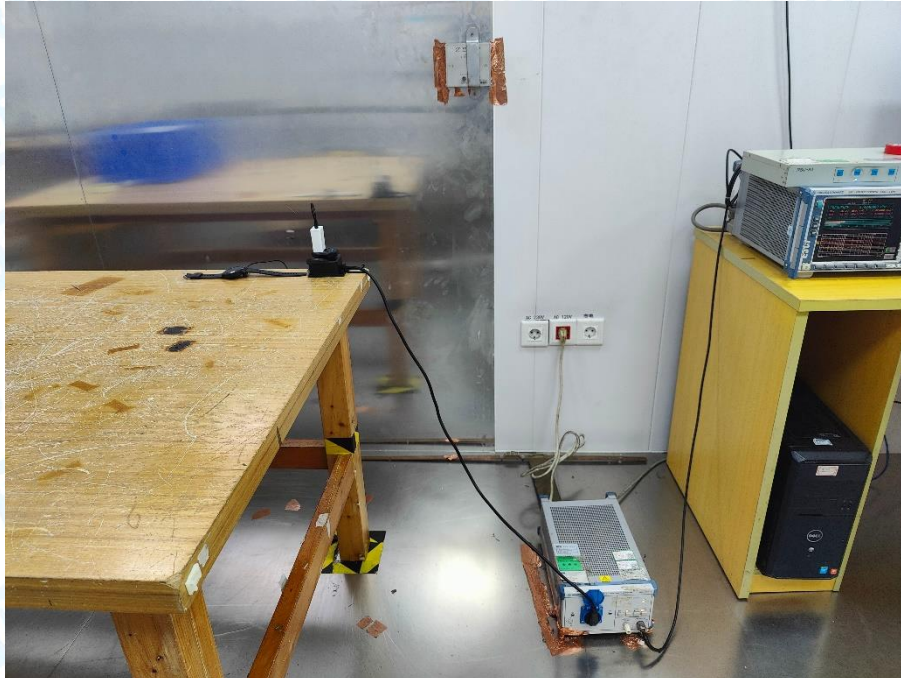
Photo of Setup for Radiated Emission (30MHz~1GHz)
