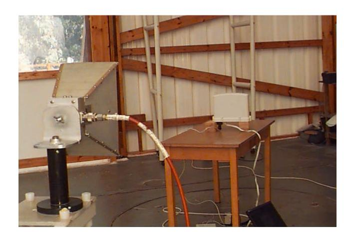
Photograph No.3 Radiated emission measurement test setup
