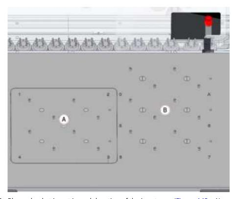
10. Place a bucket insert in each location of the input area (Figure 142 – A) and output area (Figure 142 – B), except the "0" and "A" locations of the output area. Be sure to position all bucket inserts with the positioning indicator in the right direction.
