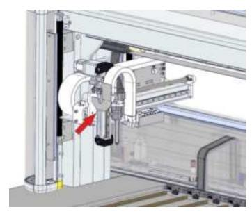
6. Clean the robot gripper with a lint-free cloth moistened with 0.1% sodium hypochlorite solution, taking care not to touch any wires, sensors, or other mechanisms.
