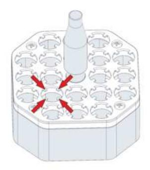
8. Place a bucket insert (Figure 135 – A) into each rotor bucket (Figure 135 – B), being sure to position all bucket inserts as shown in the figure below – see the position indicator (Figure 135 – C).
