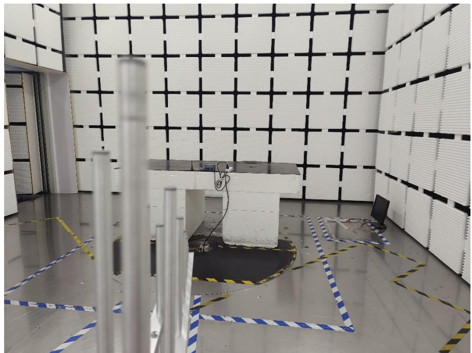
Radiation Emission Test Setup (30MHz to 1GHz)
