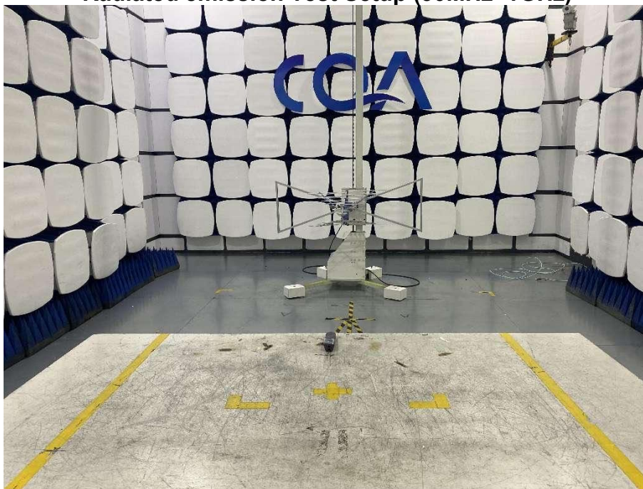
Radiated emission Test Setup (30MHz~1GHz)
