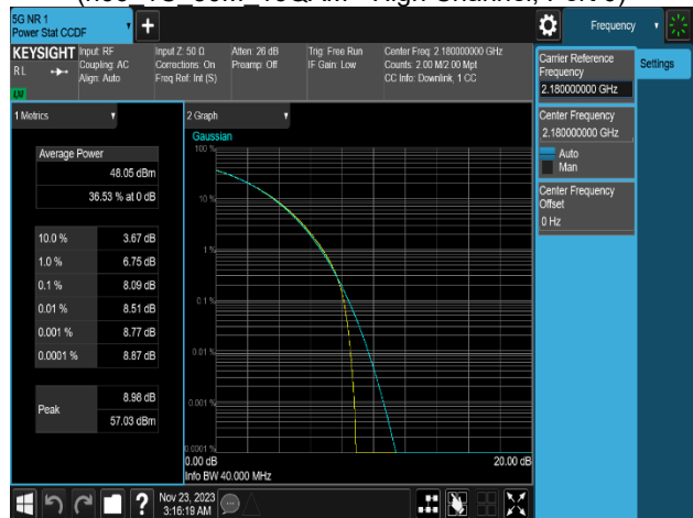
Plot 8-30. Peak To Average Power Ratio Plot (n66_3C_5M+5M+30M_QPSK - High Channel, Port 1)
