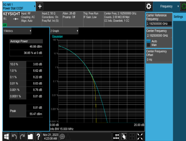
Plot 8-25. Peak To Average Power Ratio Plot (n66 1C 15M QPSK - High Channel, Port 1)
