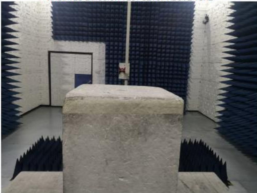
RADIATED EMISSION TEST SETUP ABOVE 1GHZ
