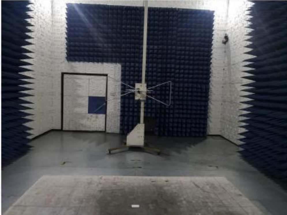
RADIATED EMISSION TEST SETUP ABOVE 1GHZ
