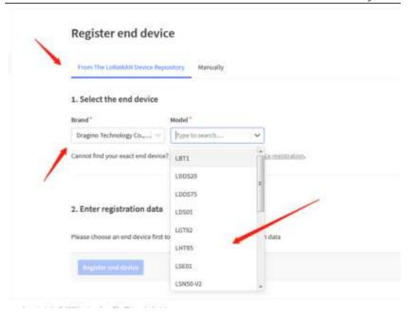
LDS02 and LDS01 use the same payload structure. So choose LDS01 as the model here.
