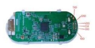
USB to TTL <- -> LDS02 RX <- -> TX TX <- -> RX
