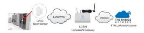
The LDS02 in installed on the door edge to detect the open / close event. And send the status to LoRaWAN server. The LDS02 will uplink two type of messages to the server.
