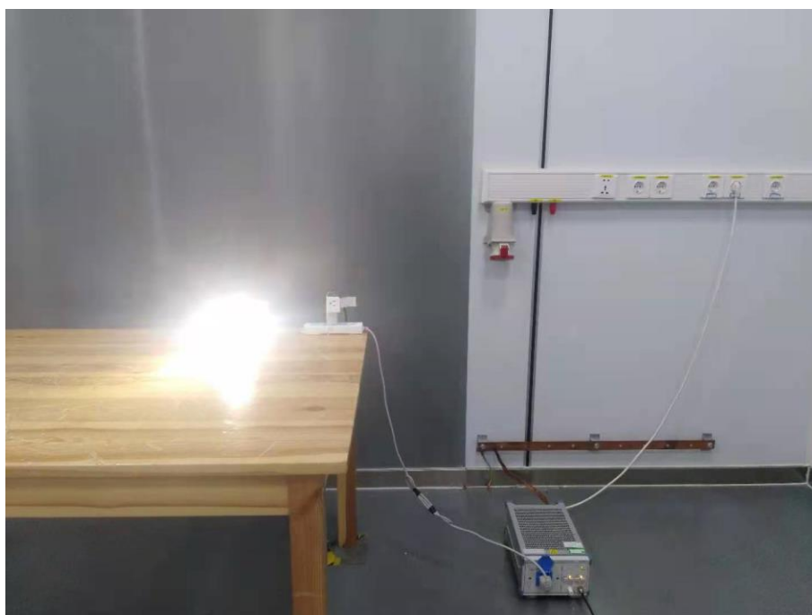
Fig. 4 Power line conducted emission setup photo
