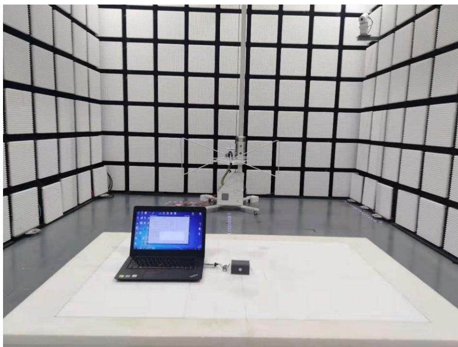
Fig. 2 Radiated emission setup photo(30MHz-1GHz)
