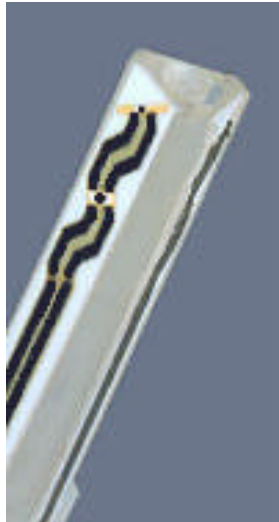
Fig. 5. ET3DV5 E-field Probe
