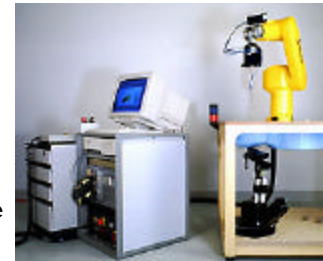
Fig. 1 SAR Test Setup
