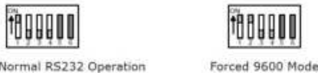
Figure 8: RS232 DIP Switch Settings (Only use Forced 9600 Mode to recover the radio when the state is unknown)
