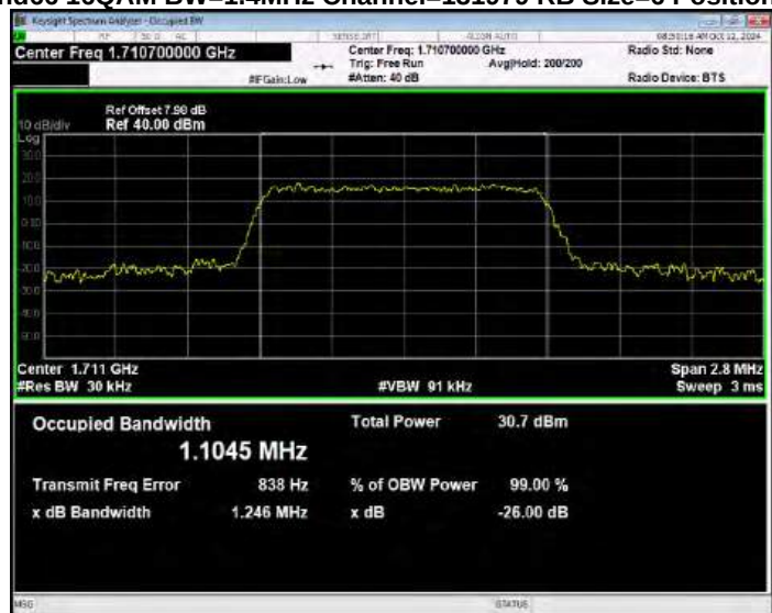
Band66 16QAM BW=1.4MHz Channel=132322 RB Size=6 Position=#0
