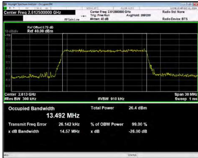
Band38 16QAM BW=20MHz Channel=37850 RB Size=100 Position=#0
