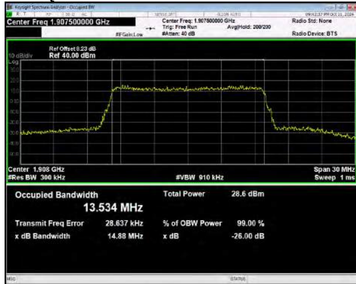
Band25 16QAM BW=20MHz Channel=26140 RB Size=100 Position=#0
