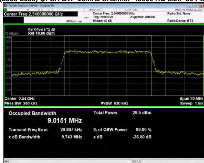
Band41(2535-2655) QPSK BW=10MHz Channel=40640 RB Size=50 Position=#0
