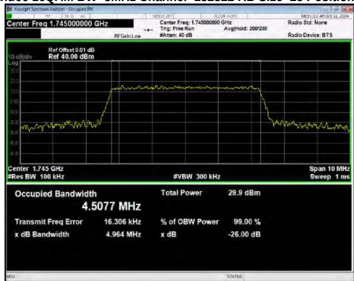
Band66 16QAM BW=5MHz Channel=132647 RB Size=25 Position=#0
