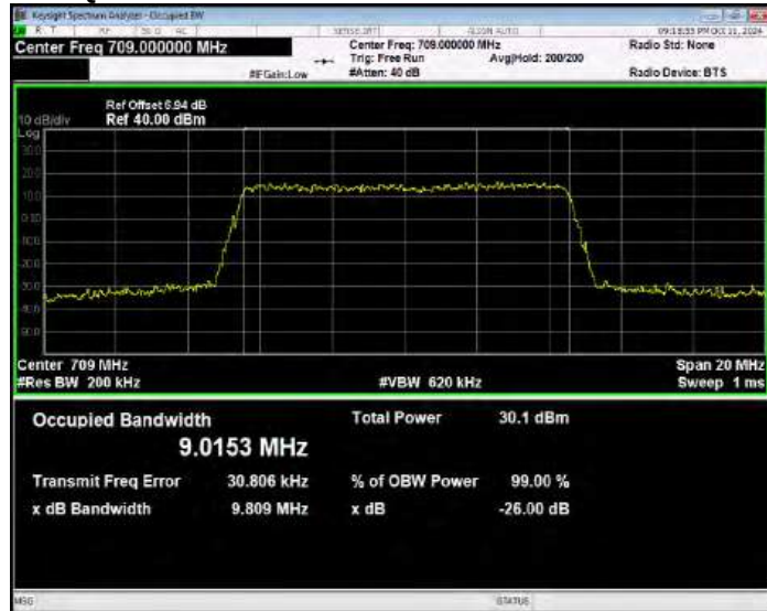
Band17 QPSK BW=10MHz Channel=23790 RB Size=50 Position=#0
