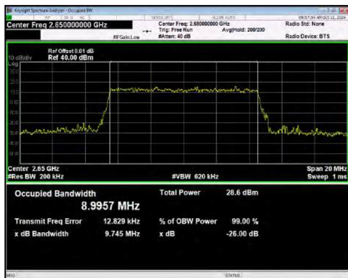
Band41(2535-2655) QPSK BW=15MHz Channel=40115 RB Size=75 Position=#0
