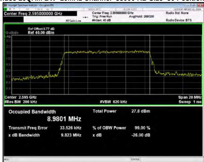
Band38 16QAM BW=10MHz Channel=38200 RB Size=50 Position=#0
