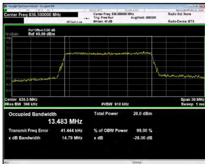
Band26(824-849) 16QAM BW=15MHz Channel=26965 RB Size=75 Position=#0
