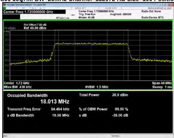
Band66 16QAM BW=20MHz Channel=132322 RB Size=100 Position=#0
