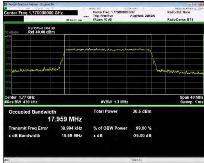
Band66 QPSK BW=3MHz Channel=131987 RB Size=15 Position=#0
