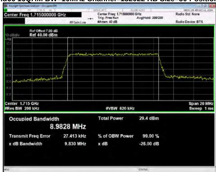
Band66 16QAM BW=10MHz Channel=132322 RB Size=50 Position=#0
