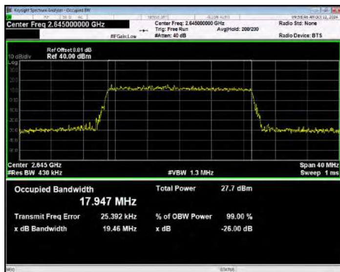
Band41(2535-2655) 16QAM BW=5MHz Channel=40065 RB Size=25 Position=#0
