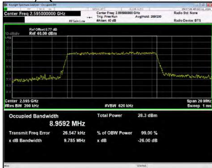
Band41(2535-2655) 16QAM BW=10MHz Channel=41190 RB Size=50 Position=#0
