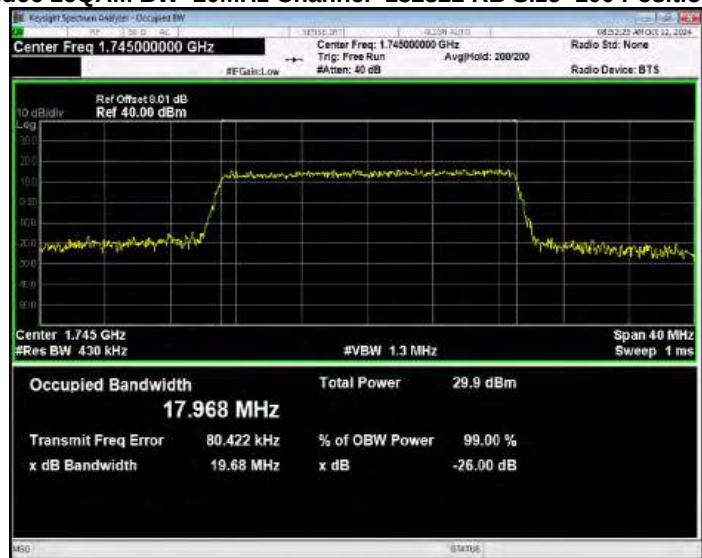
Band66 16QAM BW=20MHz Channel=132572 RB Size=100 Position=#0
