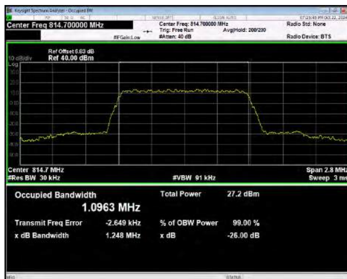
Band26(814-824) QPSK BW=1.4MHz Channel=26740 RB Size=6 Position=#0
