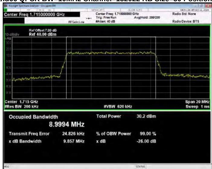
Band66 QPSK BW=10MHz Channel=132322 RB Size=50 Position=#0
