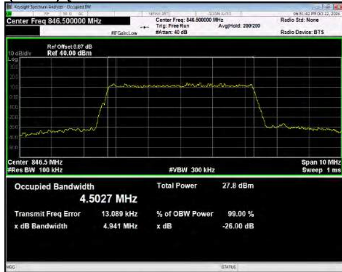
Band26(814-824) 16QAM BW=1.4MHz Channel=26697 RB Size=6 Position=#0
