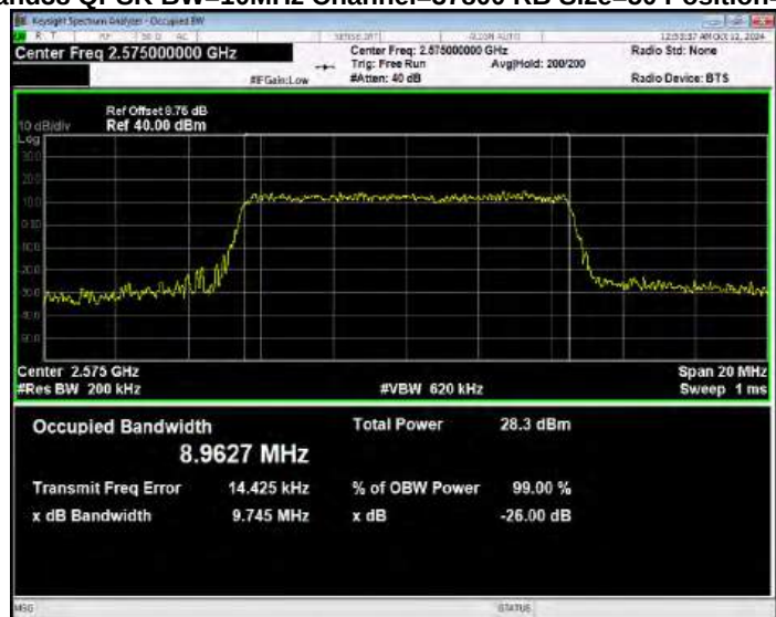
Band38 QPSK BW=10MHz Channel=38000 RB Size=50 Position=#0
