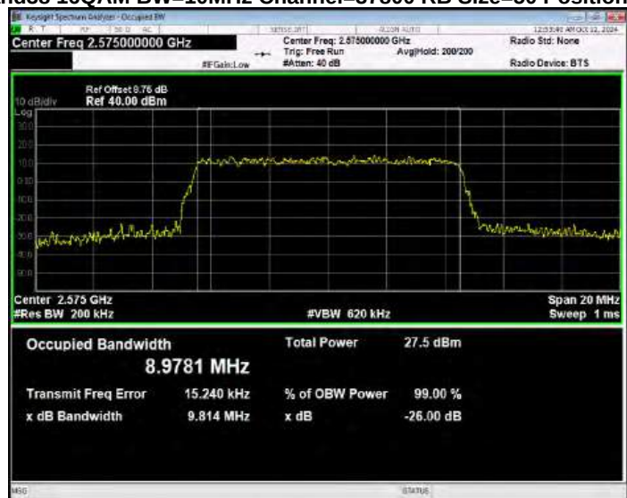
Band38 16QAM BW=10MHz Channel=38000 RB Size=50 Position=#0
