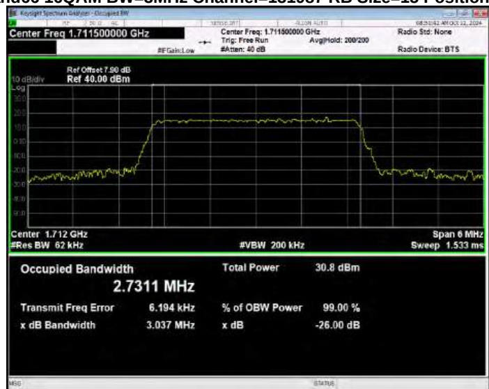
Band66 16QAM BW=3MHz Channel=132322 RB Size=15 Position=#0
