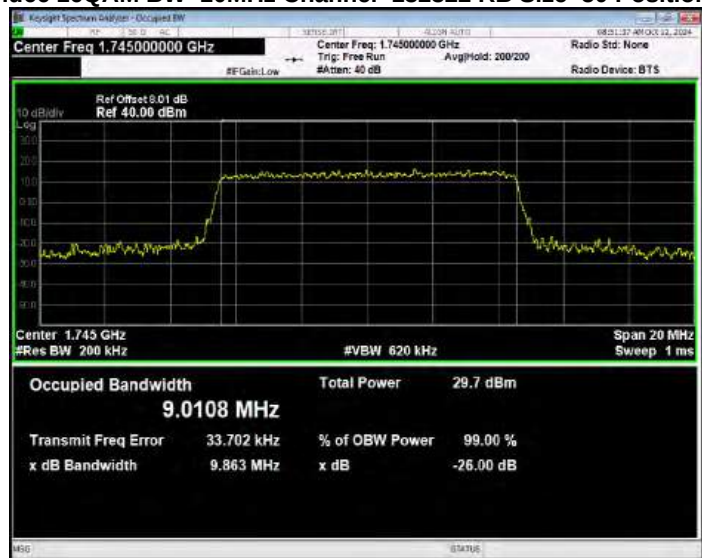
Band66 16QAM BW=10MHz Channel=132622 RB Size=50 Position=#0
