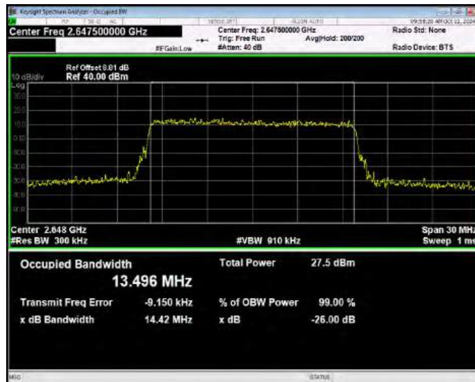
Band41(2535-2655) 16QAM BW=20MHz Channel=40140 RB Size=100 Position=#0
