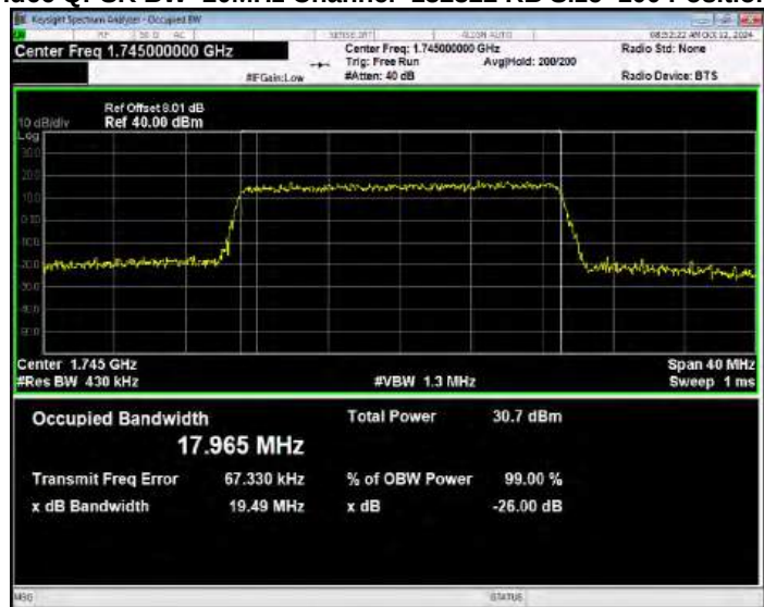
Band66 QPSK BW=20MHz Channel=132572 RB Size=100 Position=#0
