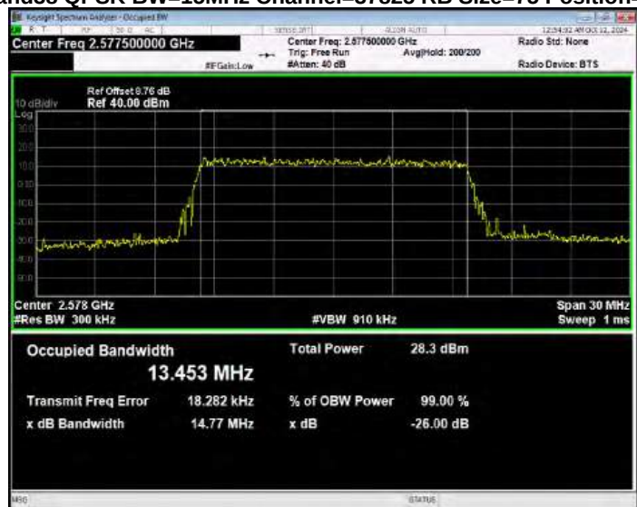
Band38 QPSK BW=15MHz Channel=38000 RB Size=75 Position=#0
