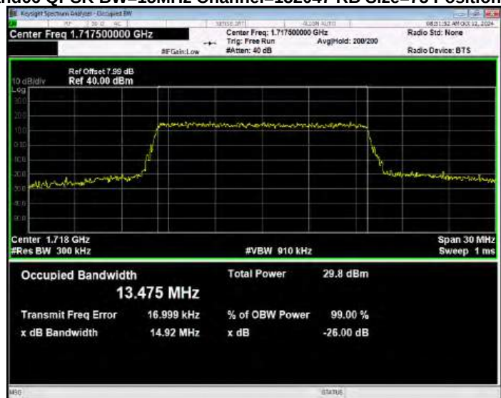
Band66 QPSK BW=15MHz Channel=132322 RB Size=75 Position=#0
