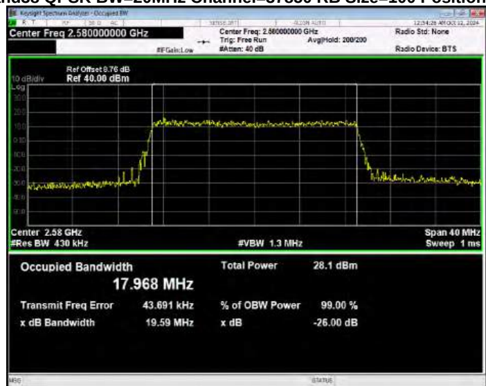
Band38 QPSK BW=20MHz Channel=38000 RB Size=100 Position=#0
