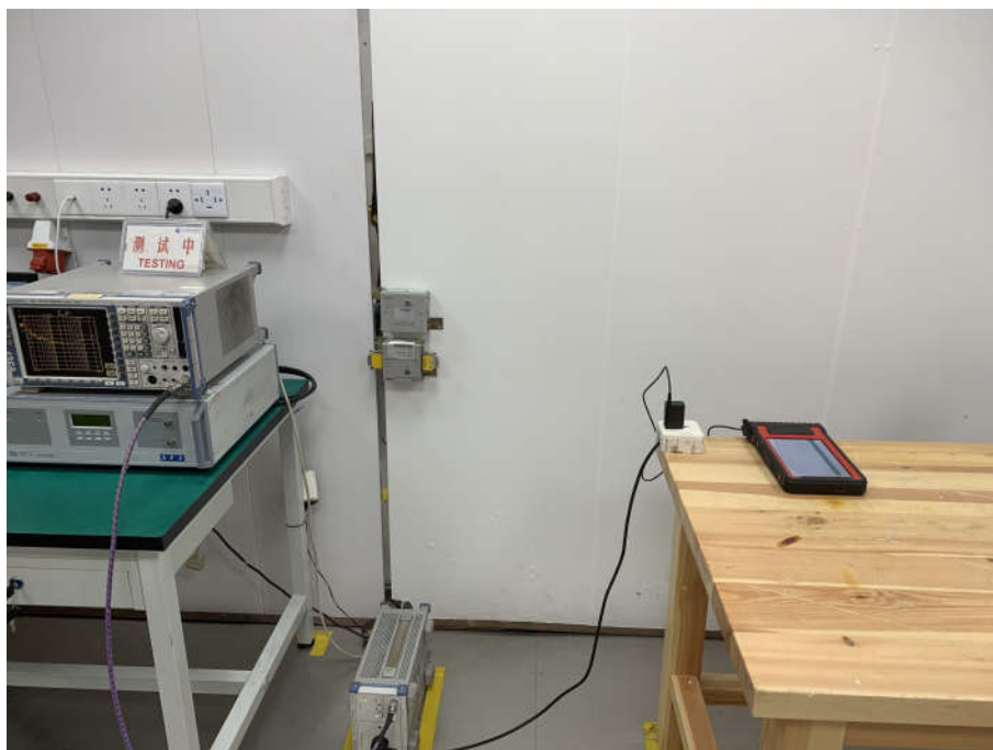
Conducted Emissions Test Setup
