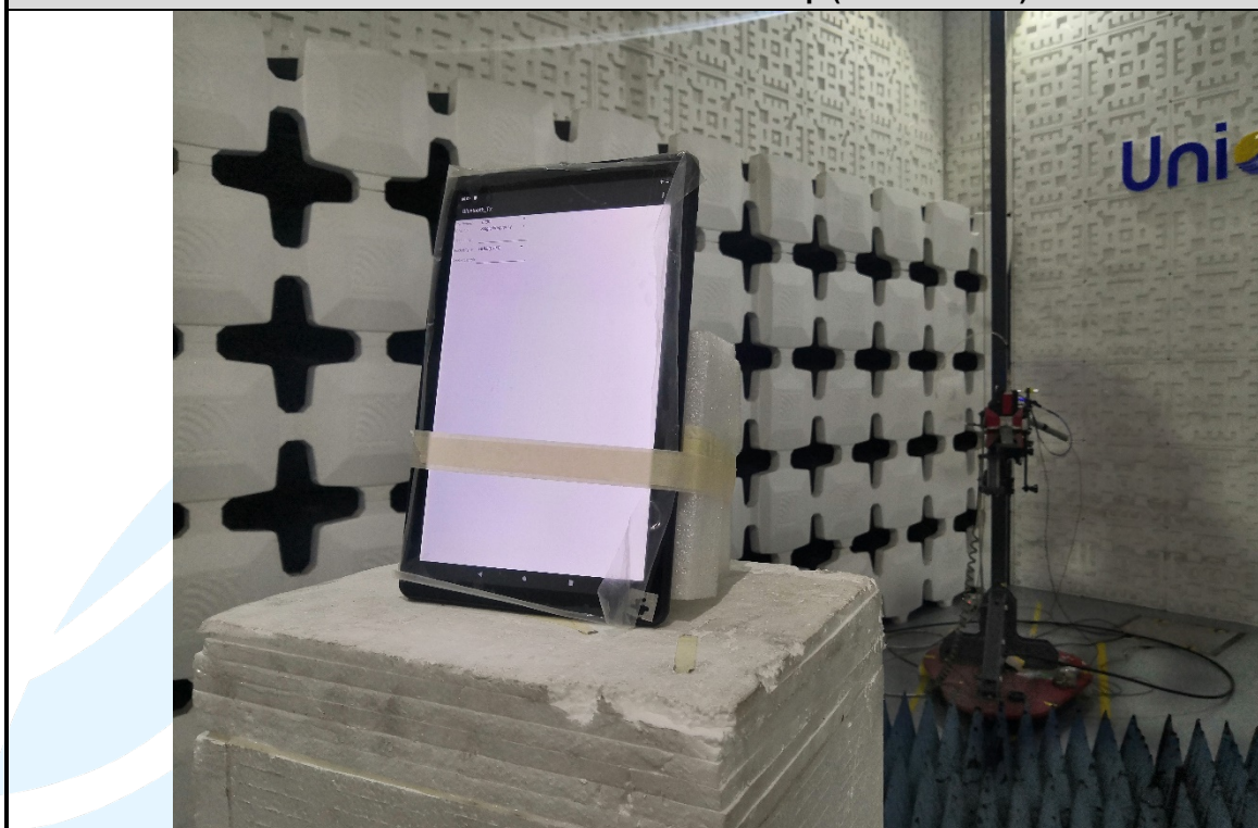
Radiated emission Test Setup (Above 1 GHz)
