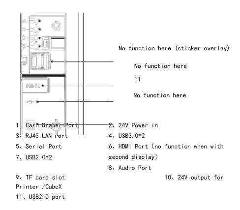
Note 1: This USB interface is only suitable for standard USB devices, such as mouse, keyboard, scanning gun, etc., and the current limit is 500mA.
