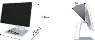
Dual-screen device, length  $\times$  width  $\times$  height. 400mm  $\times$  250mm\*370mm; the flip angle of the main screen is 0-45°, and the flip angle of the second screen is 0-30°;
